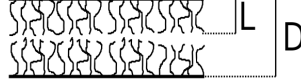
Figure 27: Alexander and de Gennes theoretical system which was used to develop the mathematical model. The system consists of two plates separated by a distance D with a layer L of grafted polymers on each.
