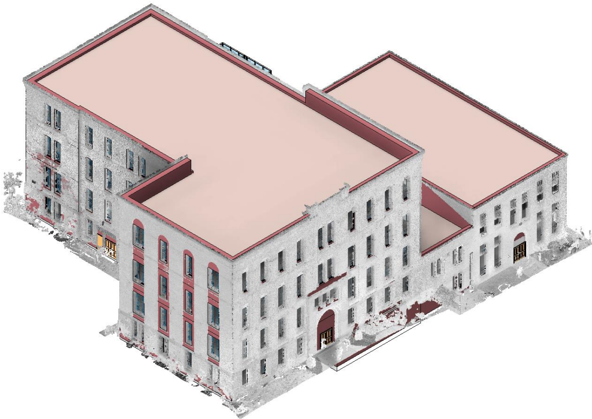
Figure 49 Sample Image of overlying the pint cloud for dimension verification
