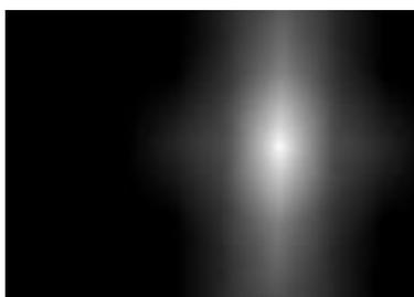
Figure 2.1: Ordinary Correlation Result Image. The magnitude of the real valued correlation function is shown as a proportional intensity in this image.
