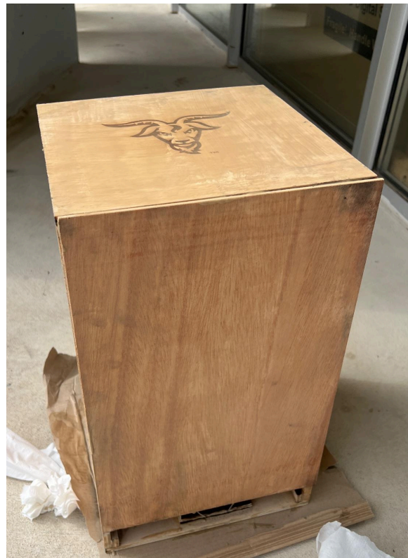
Figure 33: Completed cajón with Varnish
