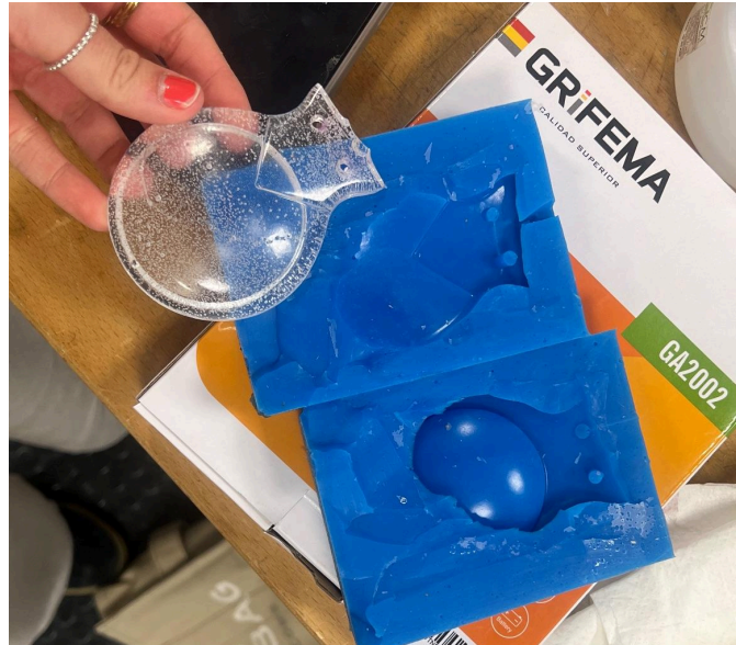
Figure 17: Resin Mold of Castanet
