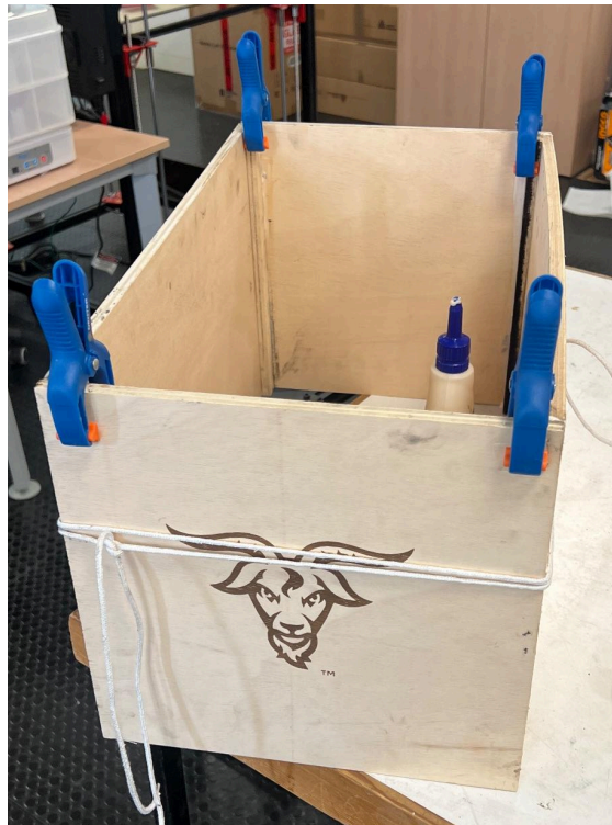
Figure 28: Top and Bottom Panel Construction
