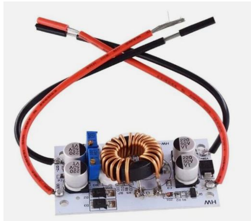
Figure 28: 4V to 40V DC Boost Converter (Ebay 2024)
