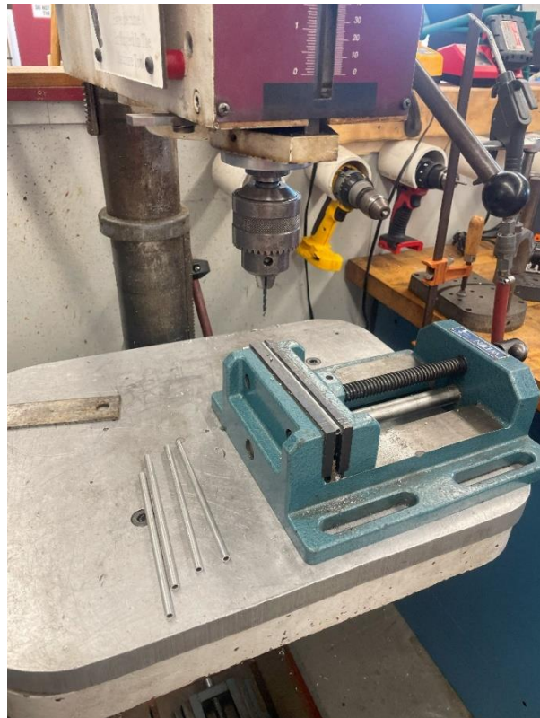
Figure 12: Drill Pressing Mounting Holes in Collectors
