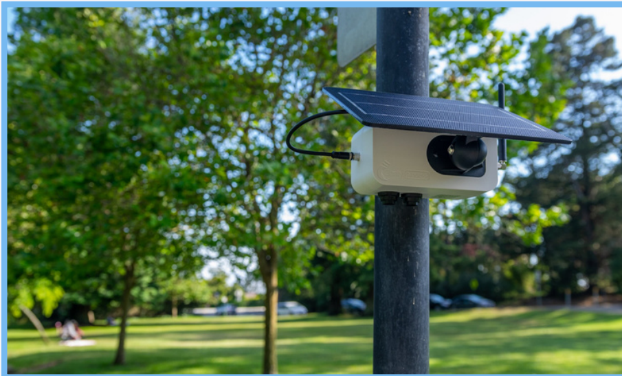
Figure 10: The air pollution monitoring node used by the Breathe London project. From: https://www.breathelondon.org/location-installation
