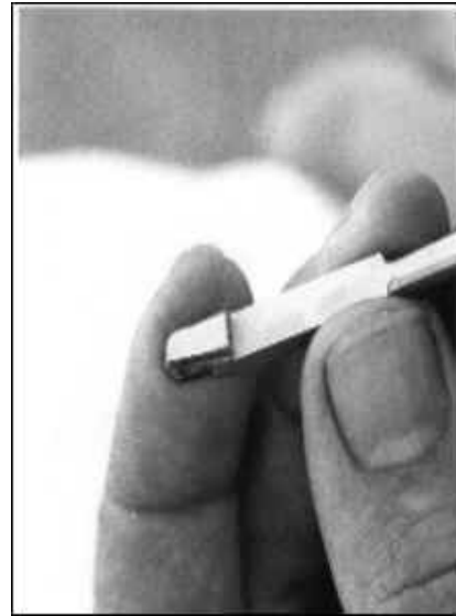
Figure 7: A Rifling-Cutter Hook 3
