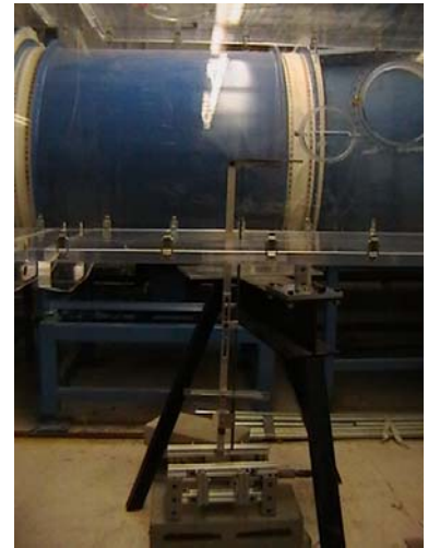
Figure 15: Drag measuring device in wind tunnel
