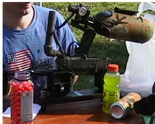
Figure 33: Paintball marker mounted in gun vice
