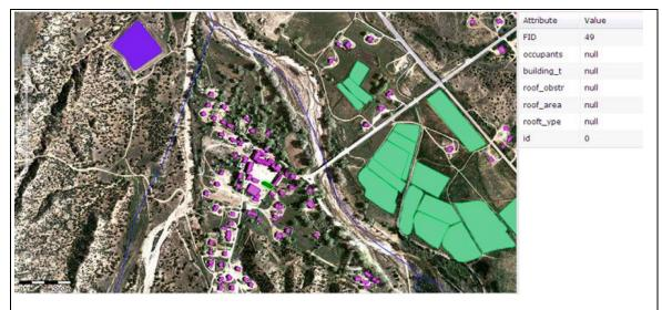
Figure 49: This map has all the shape files layered together to show the free land and attributes for each aspect. Note the attributes on the right are for the building highlighted green in the center of the map.
