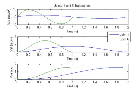
Figure 2-12: Joints 1 and 6 Trajectories
