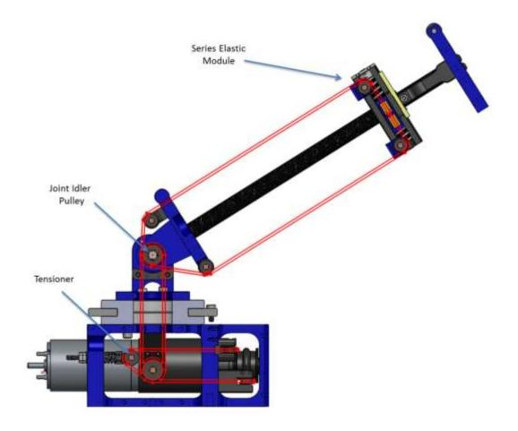
Figure 3-4: Shoulder Pivot Joint Cable Routing
