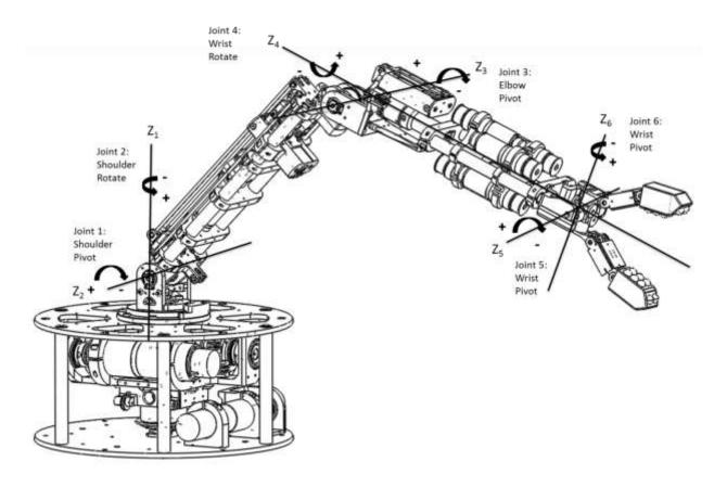
Figure 2-2: 4 DOF Arm Coordinate Axes
