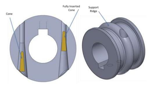
Figure 3-10: Cable Termination
