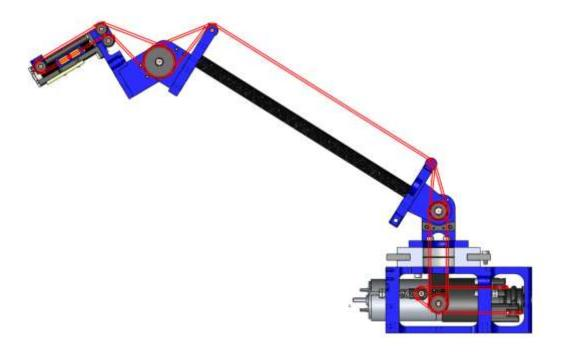
Figure 3-7: Elbow Pivot Joint Cable Routing
