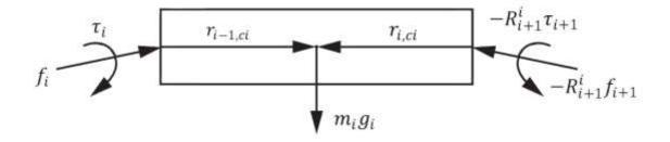
Figure 2-9: Forces and Torques on a Link [42]
