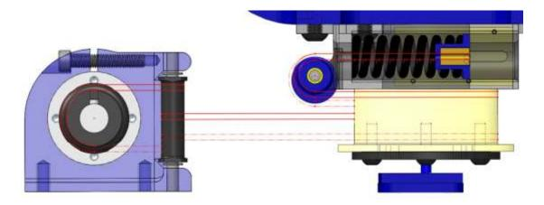
Figure 3-2: Shoulder Rotation Joint Cable Routing
