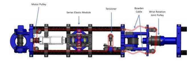
**Figure 3-9: Wrist Rotation Cable Routing**
