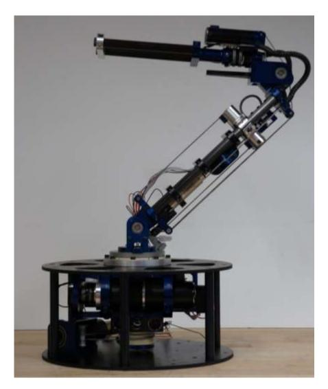
Figure 4-1: Assembled Arm
