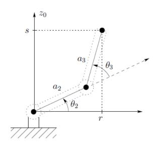
Figure 2-6: Planar Inverse Kinematics[41]
