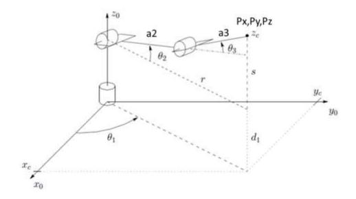
Figure 2-5: 3 DOF Elbow Manipulator Inverse Kinematics (modified from [41])
