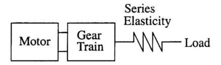
Figure 1-1: Series Elastic Actuator Block Diagram [16]
