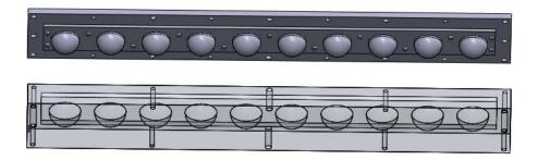
Figure 3-13: Tactile Sensor Mold
