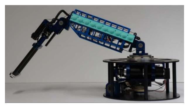
Figure 5-1: Complete First Four DOF of Robotic Arm
