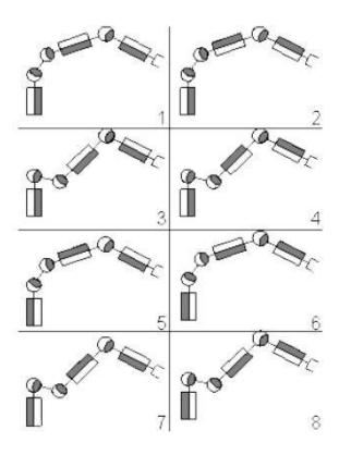
Figure 2-4: Kinematic Redundancy in an Arm [40]
