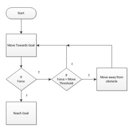
**Figure 3-15: Flowchart for Manipulation Decision Process**
