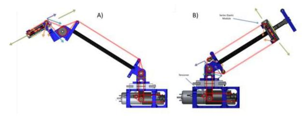
Figure 4-2: Joint Lever Arm Possibilities
