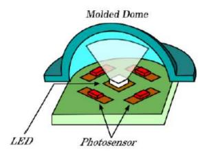
Figure 1-11: Optical Tactile Sensor [11]
