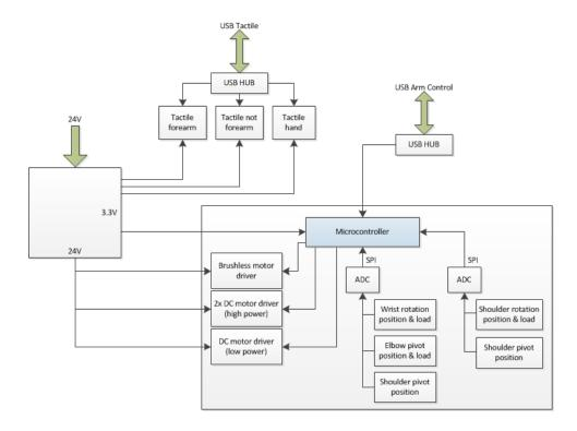
Figure 3-14: Electrical Block Diagram
