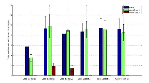
Figure 4.35 Droplet diameter changes before and after electron bombardment for all test cases (Test 1 of Case 5 not included)
