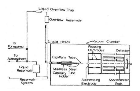
Figure 1.7 Schematic diagram of experimental setup used to generate and measure charge and velocity of liquid droplets in Hogan and Hendricks' tests [Ref. 19]
