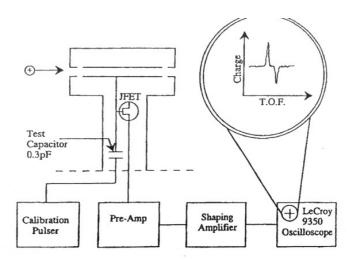
Figure 1.11 Charge detector and amplifier set up in Fuerstenau's test [Ref. 17]
