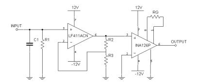
Figure 3.10 Simplified schematic of amplifier circuit [Ref. 32]
