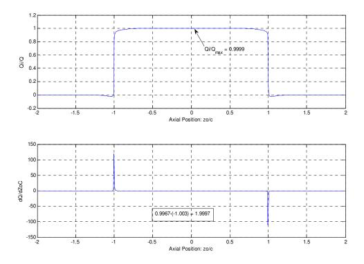
Figure 3.7 Induced charge and current for droplets travelling un-parallel to the axis of tube, droplet enters with  $\frac{r_0}{a} = -1$  and exits with  $\frac{r_0}{a} = +1$ .
