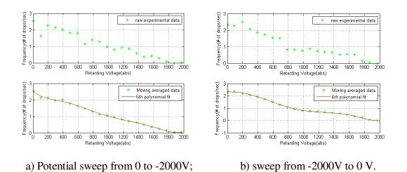
Figure 4.25 Baseline Stopping potential curve for Case 3 (Test 1),  $V_{acc} = -1723$  V.
