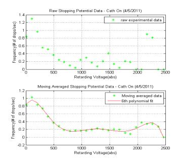
Figure 4.14 Stopping potential curve with "Cathode on" for Case 2 (Test 1) of (0 ~ -2500V),  $V_{acc 1} = -400$  V;  $V_{acc 2} = -1850$  V.
