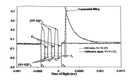
Figure 1.16 Signal induced by a charged droplet passed through the multiple stage ICD detector in Gamero-Castaño's tests [Ref. 22]
