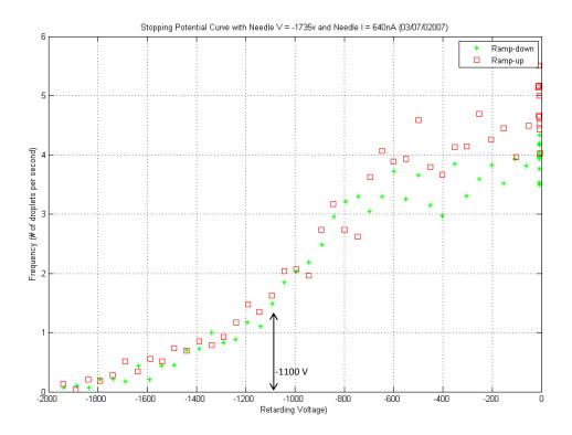
Figure 3.14 Stopping (retarding) potential curve
