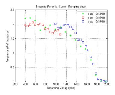
Figure 4.5 Baseline Droplet Stopping potential curve with a sweep range of -400~ -2000 V,  $\Delta V = -50$  V,  $\Delta t = 600$  S.
