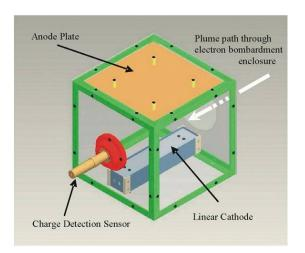
Figure 3.16 CAD drawing of CDMS/Thermionic cathode with anode plate
