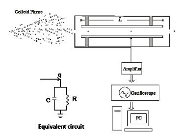
Figure 3.4 Schematic of the induced charge sensor
