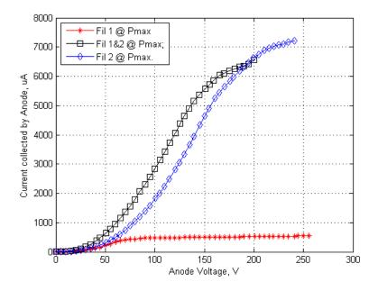
Figure 4.1 Measured anode current  $I_{an}$  as a function of anode voltage  $V_{an}$ , with no electrospray
