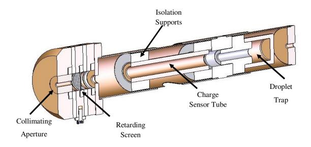
Figure 3.9 Cutaway drawing showing CDMS mechanical layout
