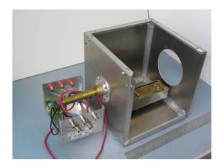
Figure 3.17 Picture of CDMS/Thermionic cathode without anode plate
