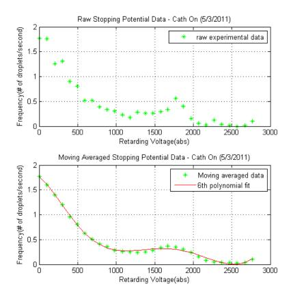
Figure 4.7 Typical stopping potential for droplets subjected to electron flux, with a sweep range of 0 to -2800 V, with  $\Delta V$ =-100 V,  $\Delta t$ =90 sec. (Test 1 of Case 4)
