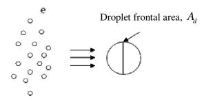
Figure 2.4 Conceptual diagram showing electrons collected by negatively charged droplet
