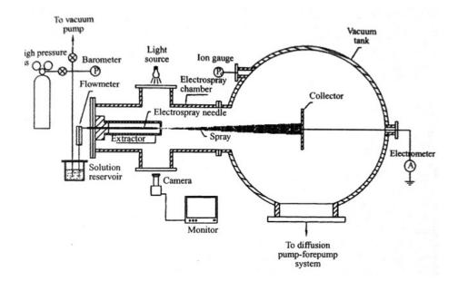
Figure 1.12 Electrospray source and vacuum facility in Gamero-Castaño's tests [Ref. 21]
