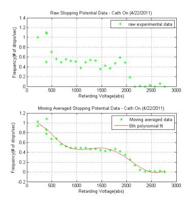
Figure 4.26 Stopping potential curve with "Cathode on" for Case 3 (Test 1) of (0 to -2800V),  $V_{acc1} = -450$  V;  $V_{acc2} = -2100$  V.
