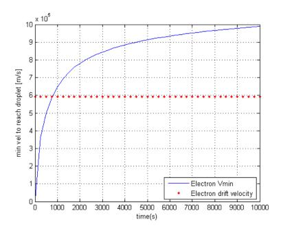
Figure 2.6 Negatively charged droplet charges up with  $V_{an} = 1 \text{ V} (v_{\min} \text{ vs. } t)$
