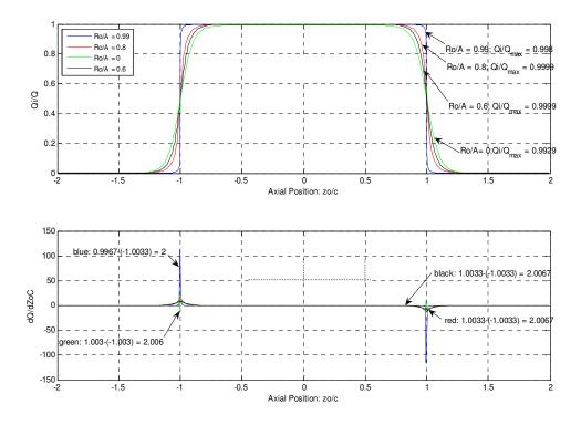
Figure 3.6 Induced charge and current for droplet travelling parallel to the tube axis, with an (trajectory) axis ratio of 0.99, 0.8, 0.6 and 0
