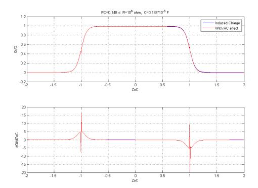
Figure 3.8 Effect of the measuring electronics on induced charge and current
