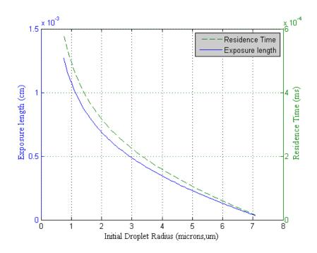
Figure 2.2 Exposure length and residence time (to reach Rayleigh limit) as a function of droplet radius.
