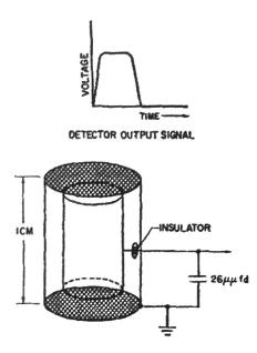
Figure 1.3 Shelton's single sensing tube detector [Ref. 16]
