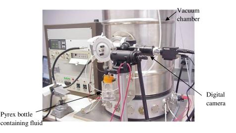
Figure 3.1 Facility used for electrospray including the vacuum chamber, Pyrex bottle containing fluid and digital camera to monitor the Taylor cone and jet.
