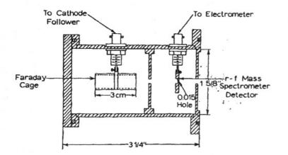
Figure 1.8 Schematic diagram of Faraday cage detector used to measure individual particle charge and velocity in Hogan & Hendricks tests [Ref. 19]
