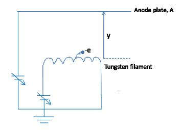
Figure 2.1 Conceptual diagram for electron energy balance
