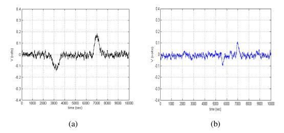
Figure 4.6 Typical waves captured by CDMS, with droplets subjected to electron flux
