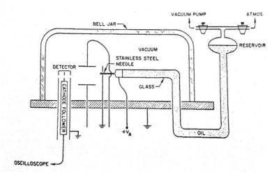
Figure 1.6 Schematic of experimental set up for Hendricks' tests [Ref. 18]
