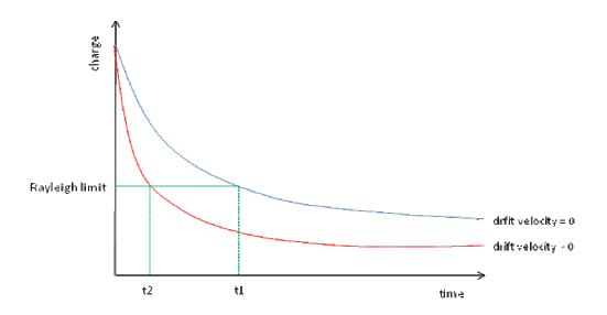
Figure 2.3 Conceptual diagram of charging process with and without electron drift velocity
