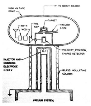
Figure 1.5 Experimental setup used by Shelton to accelerate iron powder particles [Ref. 16]
