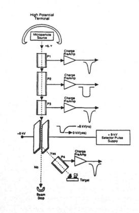
Figure 1.9 General scheme for producing and detecting electrostatically charged microparticles with high velocity in Keaton's tests [Ref. 20]
