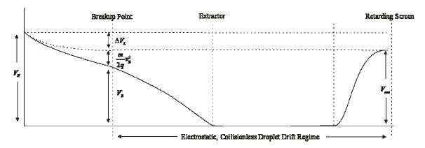
Figure 3.13 Acceleration Potential Mechanism Scheme
