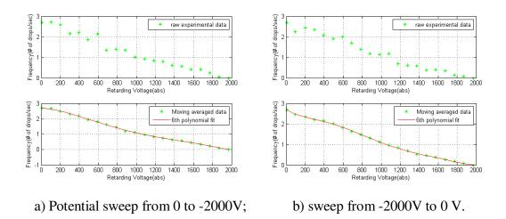
Figure 4.29 Baseline Stopping potential curve for Case 4 (Test 1),  $V_{acc} = -1700$  V.
