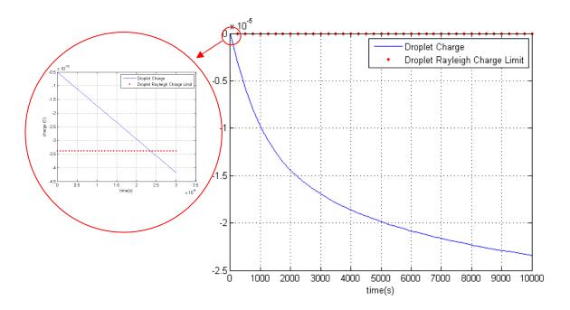
Figure 2.5 Negatively charged droplet charges up with  $V_{an} = 1V(q \text{ vs. } t)$
