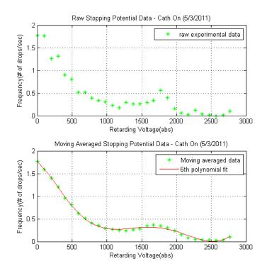
Figure 4.30 Stopping potential curve with "Cathode on" for Case 4 (Test 1) of (0 to -2800V),  $V_{acc1} = -500$  V;  $V_{acc2} = -2050$  V.
