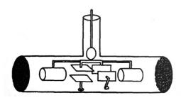
Figure 1.4 Shelton's charge-velocity-position detector [Ref. 16]
