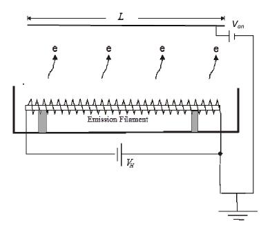
Figure 3.15 Diagram of thermionic cathode with accelerating anode plate
