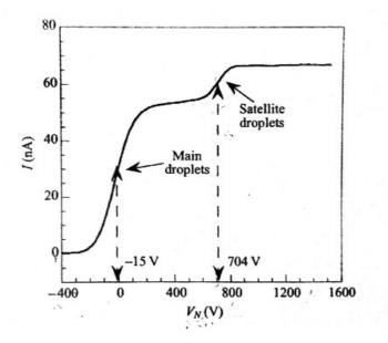
Figure 1.13 Typical stopping potential curve for electrospray in Gamero-Castaño's tests [Ref. 21]
