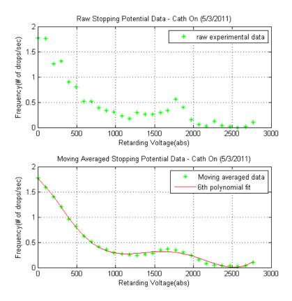
Figure 4.22 Stopping potential curve with "Cathode on" for Case 2 (Test 3) of (0 to -2800V).  $V_{acc 1} = -450$  V;  $V_{acc 2} = -1900$  V.
