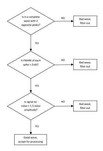
Figure 4.3 Criterion for Preliminary selection of "good" waves. ( $\Delta t = 4 \times 10^{-7}$ s, which is the time step used in CDMS capture vi showing the frequency of data capture)
