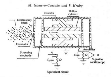
Figure 1.14 Schematic of capacitive detector used by Gamero-Castaño to measure charge and specific charge of electrospray droplets [Ref. 21]
