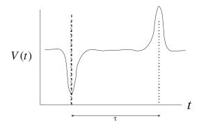
Figure 3.12 Diagram of induced voltage trace on the sensor tube indicating the time-of-flight (TOF) as the distance between pulse peaks.
