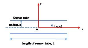
Figure 3.5 Schematic of droplet location in the sensor tube
