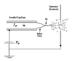
Figure 1.2 Diagram of colloidal electrospray source
