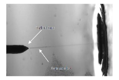
Figure 3.3 Photograph of electrospray operating at  $V_n$ =1688 V,  $I_n$ =52 nA and  $P_c$ =7.1×10<sup>-5</sup> Torr.
