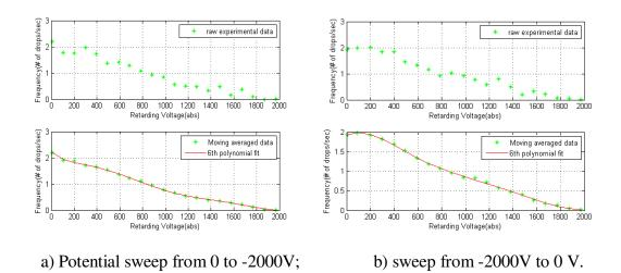
Figure 4.21 Baseline Stopping potential curve for Case 2 (Test 3),  $V_{acc} = -1622$  V.
