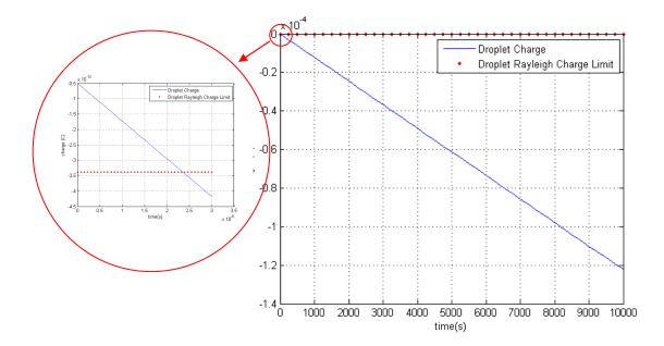
Figure 2.7 Negatively charged droplet charges up with  $V_{an}$  =20 volts (q vs. t)
