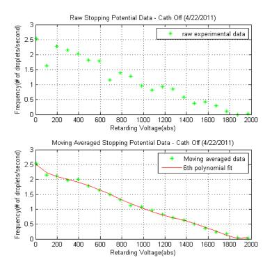
Figure 4.4 Typical baseline Droplet Stopping potential curve with a sweep range of 0 to -2000 V, with  $\Delta V = -100$  V,  $\Delta t = 30$  sec.
