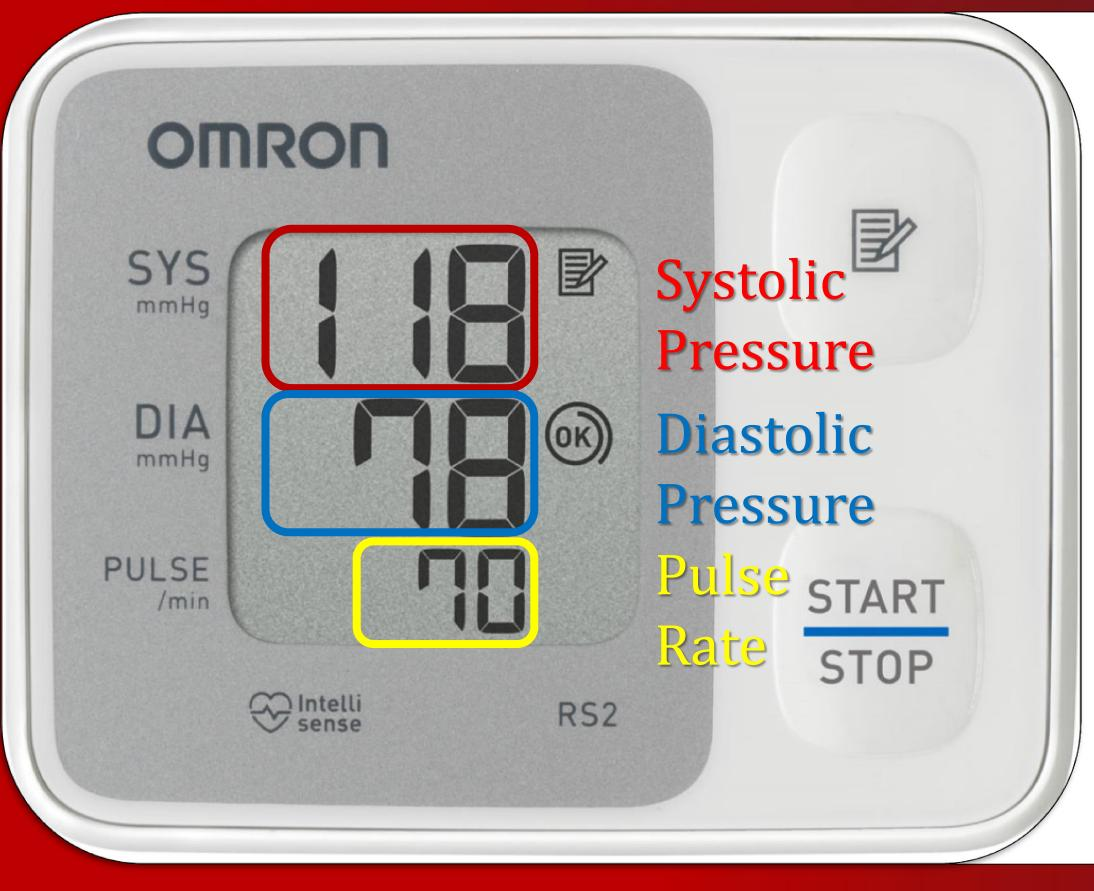
The screen of one type of electronic blood pressure monitor
