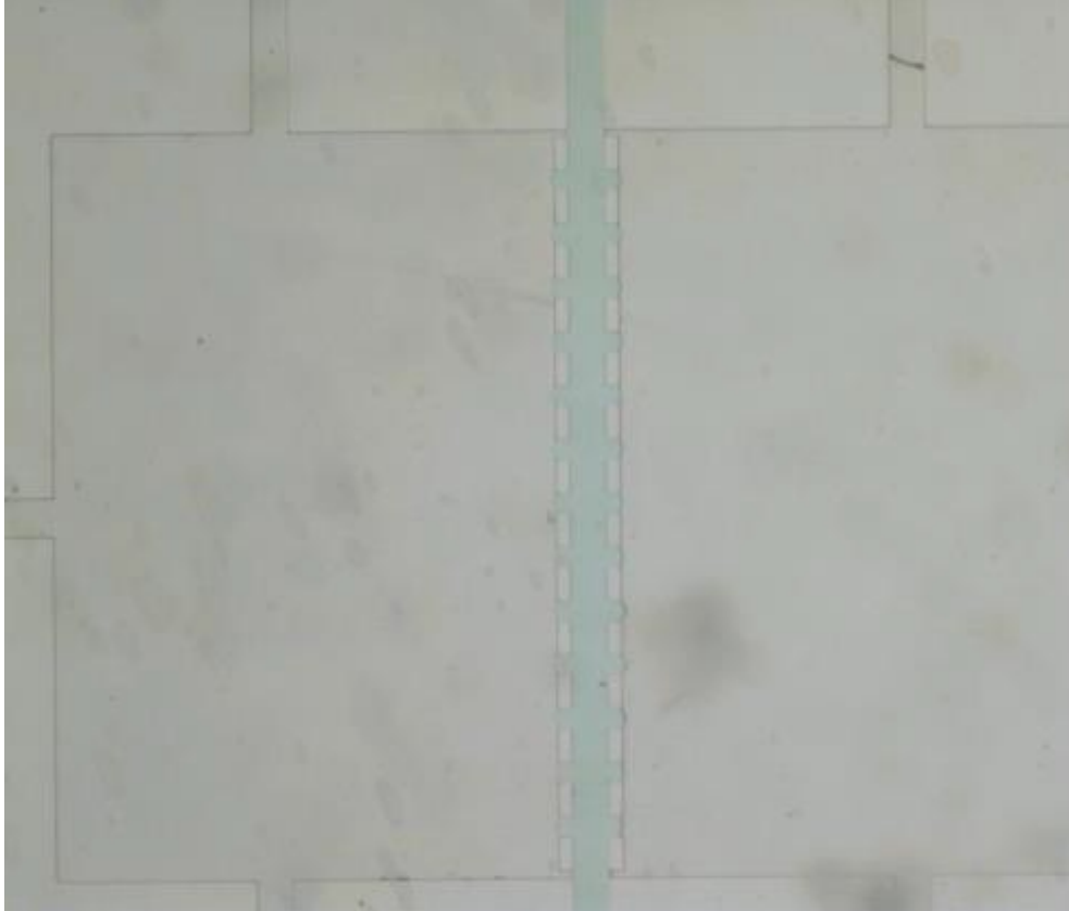
Figure 4.9 – 4mm Device Model of Hydrogel Barrier Using Water and Green Dye
