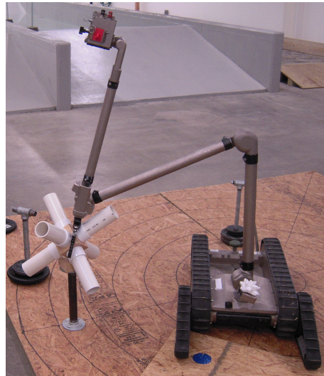
Fig. 1. The iRobot PackBot, a robot with its 5-DOF, picking up an object.
