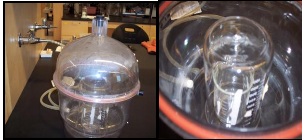
Figure 5: Vacuum infiltration set up, viewed from the outside; detailed view from the inside
