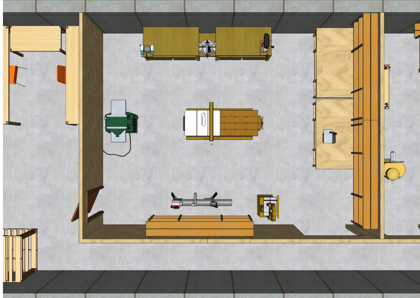
Figure 2.9. Woodshop design showing table saws, a drill press, a lathe, a band saw, a sander, and a wood planer. This layout is about 24 feet wide by 20 feet long.
