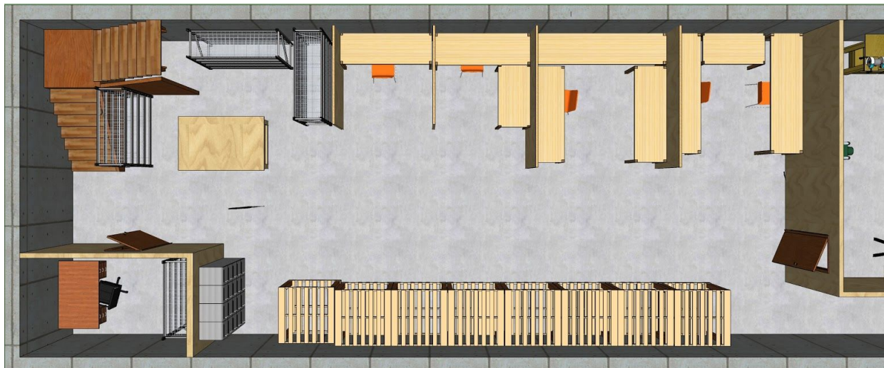
Figure 2.8. Storage and Extra Office Space design. This area must first accomplish the task of storing materials and member projects and personal items. Shelving is shown near the stairs for material and tool storage. Lockers are near the bottom left wall and pallets are along the bottom wall for rental storage. A small office was made for the facilities manager and all remaining space could be used for cubical space.
