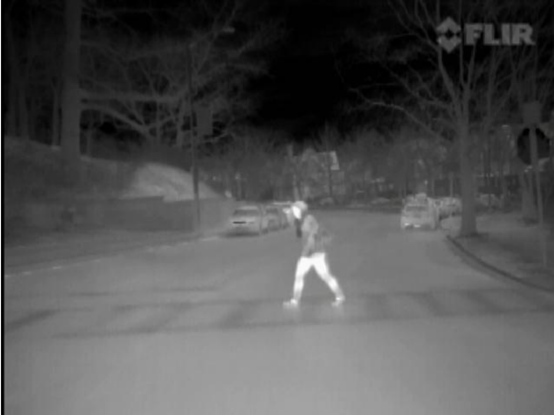
Figure 4.8: Sample thermal image of LWIR camera
