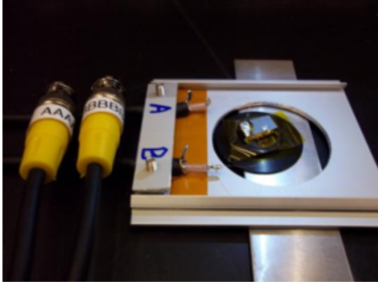
Figure 27: The sample holder used for the NSOM experiment. The wires are connected to BNC cable by indium solder.
