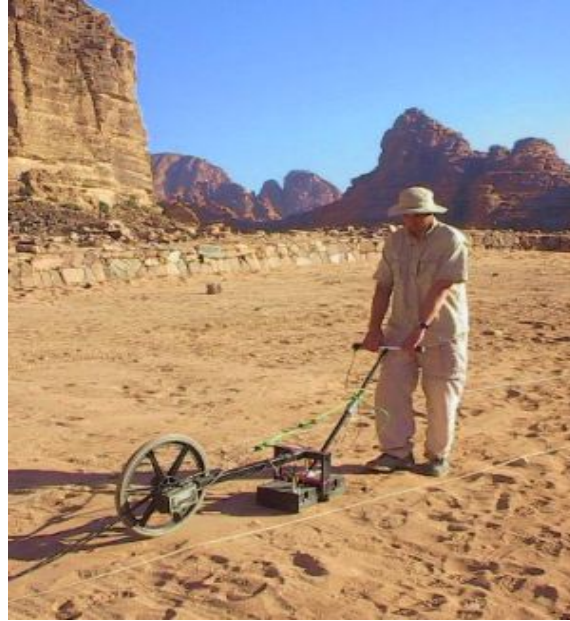
Figure 4: A man conducting site work using survey lines and a ground penetrating radar [6]
