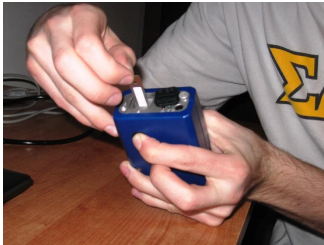
Figure 91: Changing the Aethalometer's Filter
