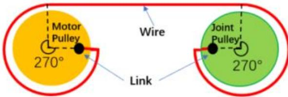
Figure 2.1: The connection between the wire, actuator, and joint (Source: Li et al., 2018).
