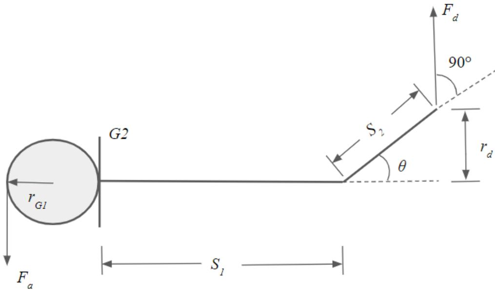
Figure 4.7: Schematic for the Static Force Analysis of the Shoulder Roll DOF.
