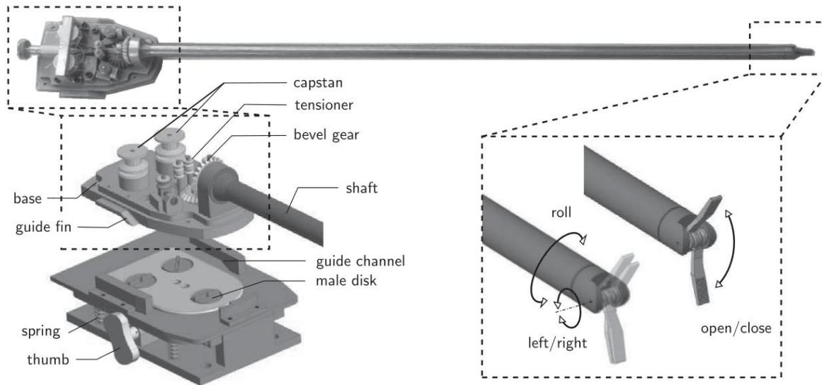
*Figure 1.2: A 3 Degrees of Freedom Model of a MIRS Tool (Source: Nisar et al., 2020).*
