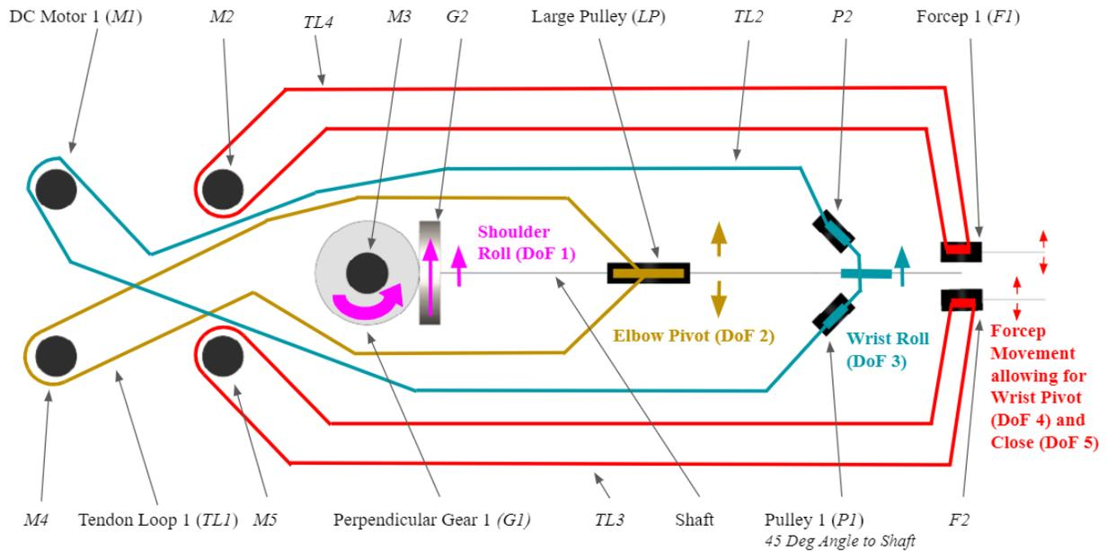
Figure 4.5: Actuation of Each DoF.
