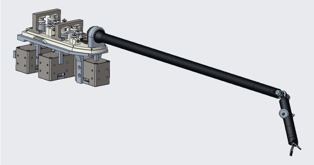
*Figure 4.11: An image of the CAD of the 5-DoF Surgical Tool. The forceps are separated in the image to show their ability to move, allowing for the close DoF. Similarly, the elbow pivot and shoulder roll DoFs are utilized in the image to create a larger surgical workspace.*
