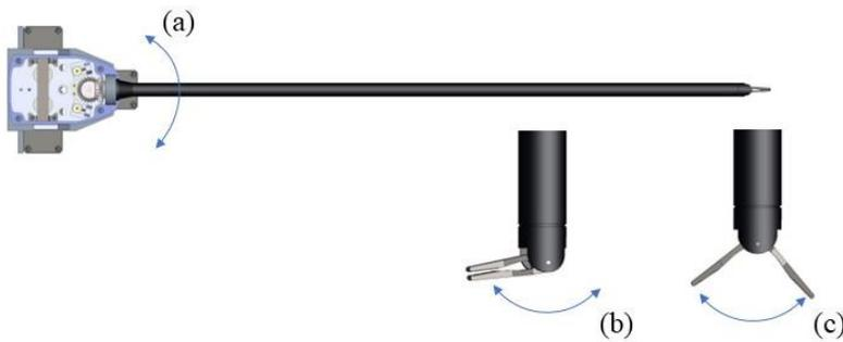
Figure 2.7: Three degrees of freedom in the current surgical tool.
