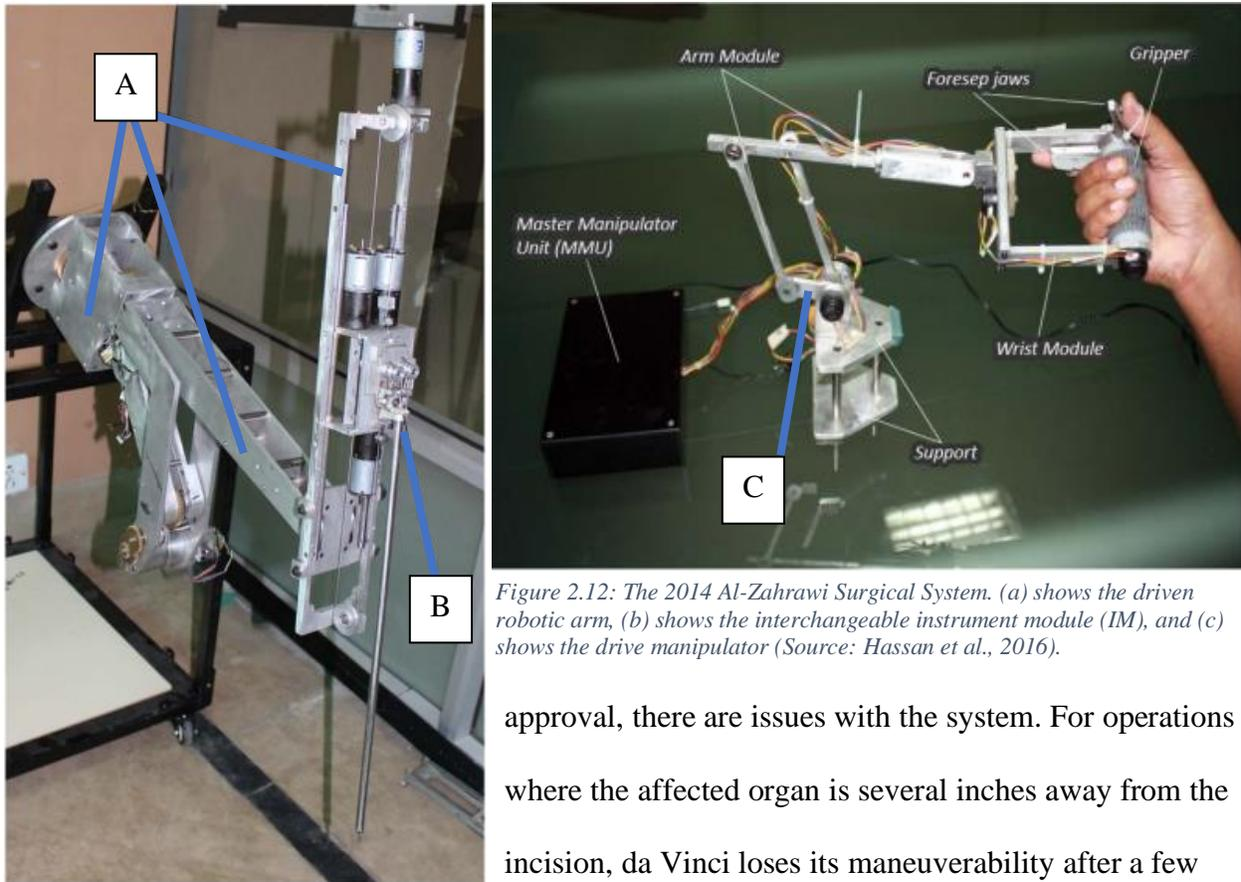
Figure 2.12: The 2014 Al-Zahrawi Surgical System. (a) shows the driven robotic arm, (b) shows the interchangeable instrument module (IM), and (c) shows the drive manipulator (Source: Hassan et al., 2016).
