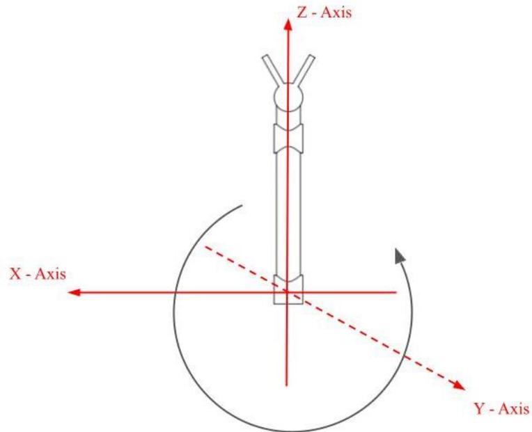
*Figure 4.2: Diagram of X-Z Movement in the DoF Layout Utilizing Two Rotational Joints. In the diagram, the origin is set at the center of the elbow joint. The portion of the tool shown is the section between the elbow joint and the end of the forceps.*
