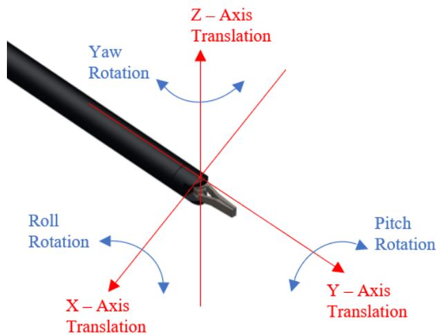
Figure 3.1: DoF Considerations of Wrist on a 3-D Coordinate Plane.
