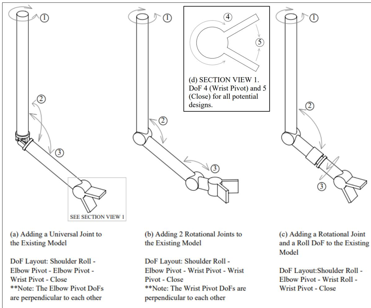
Figure 4.3: DoF Layouts Considered for the Realized Design.
