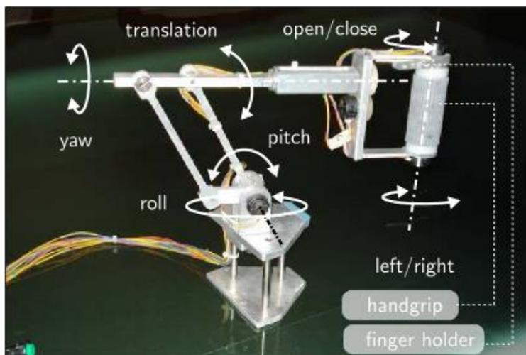
Figure 2.3: The drive manipulator in the (Nisar et al., 2020) model.
