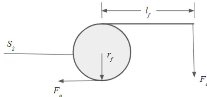
Figure 4.10: Schematic for the Static Force Analysis of the Forceps.
