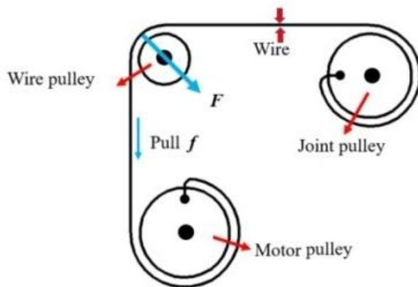
Figure 2.2: Tendon connected to multiple pulleys (Source: Li et al., 2018).
