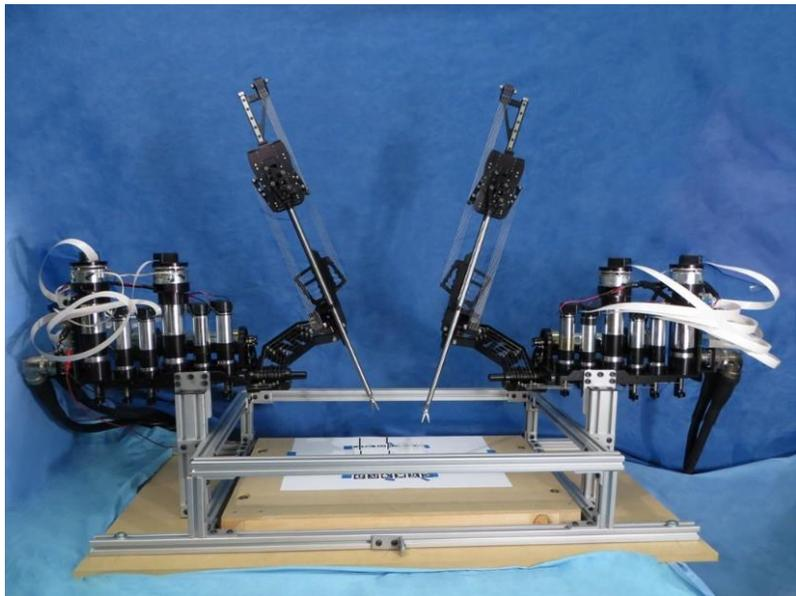
*Figure 2.9: Raven II Surgical System (Source: Raven II - ROBOTS, n.d.).*
