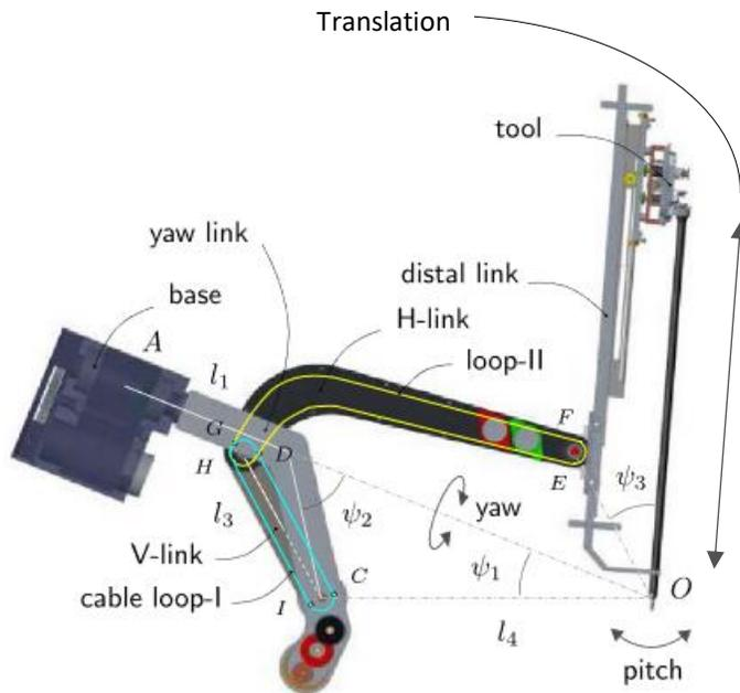
Figure 2.4 The driven manipulator (robotic arm) in the (Nisar et al., 2020) model.
