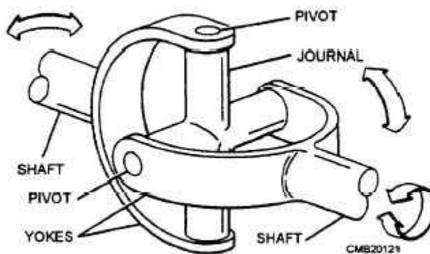
*Figure 4.1: The Universal Joint. The cross within the joint is formed by the perpendicular intersection of the two journals at the center of the joint (Source: Cross and Roller Universal Joint, n.d.)*
