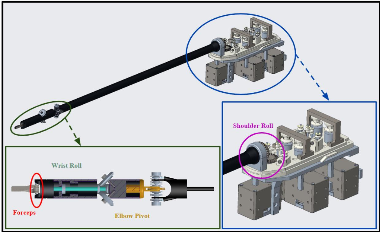
Figure 4.4: A Three-Dimensional View of the CAD of the Realized Model. Actuated by 5 servomotors, it utilizes tendons and gears to attain five degrees of freedom (DoF): shoulder roll, elbow pivot, wrist roll, wrist pivot, and close. The sectioned views show the mechanical elements of how different components of the tool move.
