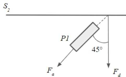
Figure 4.9: Schematic for the Static Force Analysis of the Wrist Roll DOF.
