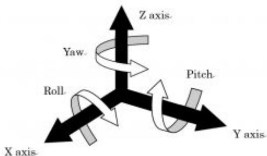
Figure 2.5: Illustration of the six degrees of freedom (Source: Mechanism of 6 Degrees of Freedom Vibration Test System, 2017).
