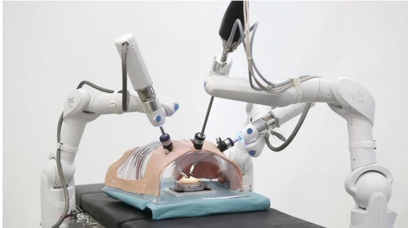
*Figure 2.8: MicroSurge Surgical System (Source: DLR - Institute of Robotics and Mechatronics - MiroSurge, n.d.).*
