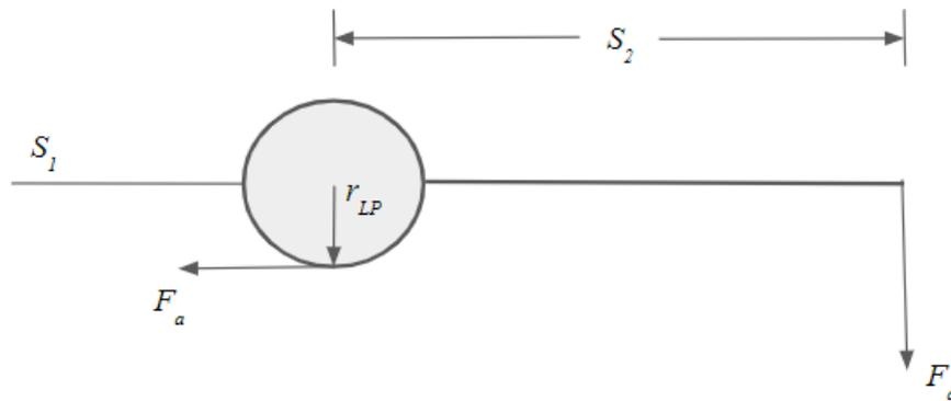
Figure 4.8: Schematic for the Static Force Analysis of the Elbow Pivot DOF.
