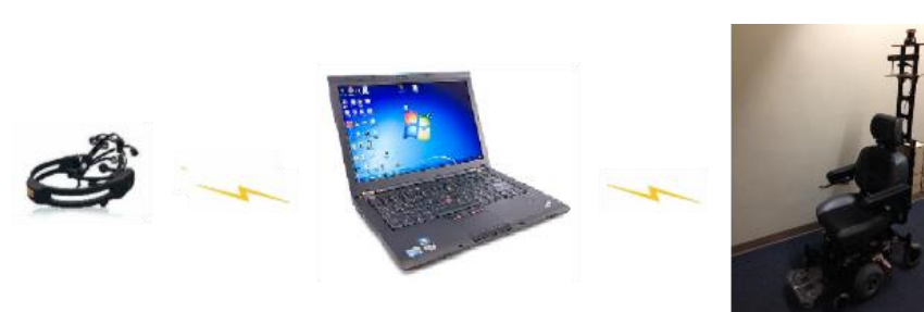
Figure 5: Communication among Emotiv headset, computer, and wheelchair
