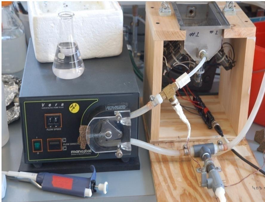
Figure 3-2: Harris Acoustic Products flow through sonication system
