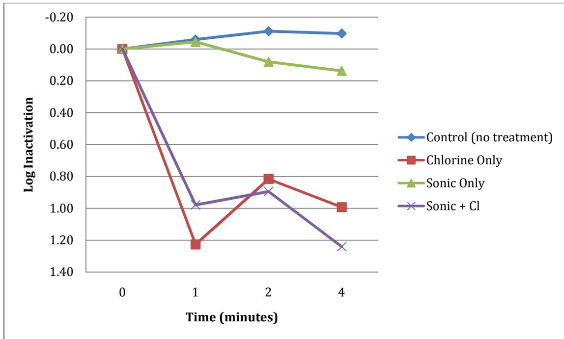
Figure 4-3: Log inactivation of *E. coli* with cavitation chamber system (performed at Tufts)
