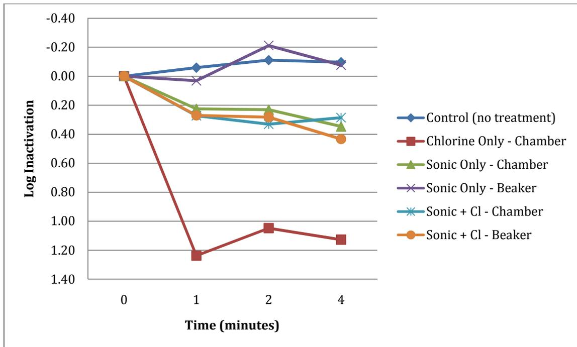
Figure 4-1: Log inactivation of *E. coli* with probe sonication system (performed at Tufts)
