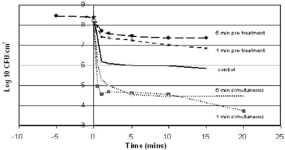
Figure 2-2: Chlorine inactivation of *E. coli* with pre- and simultaneous sonication at 20 kHz (Duckhouse, *et al.* 2004)
