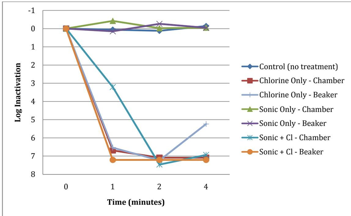
Figure 4-2: Log Inactivation of *E. coli* with Probe Sonication System (performed at WPI)
