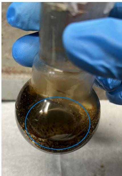
Figure 5: Water Bubble formed on top of bio-oil from the 325 C trial
