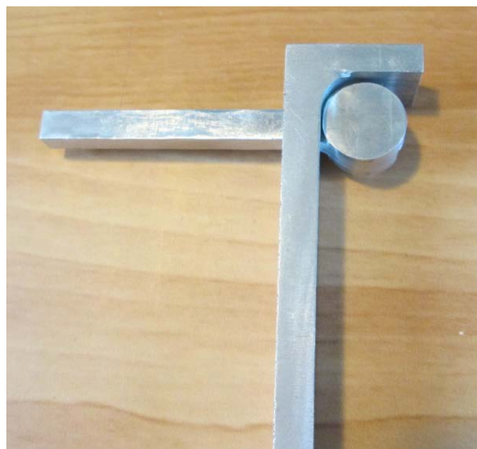
Figure 13: Second prototype of hinge made in the machine shops at Wasburn Labs using Aluminum.
