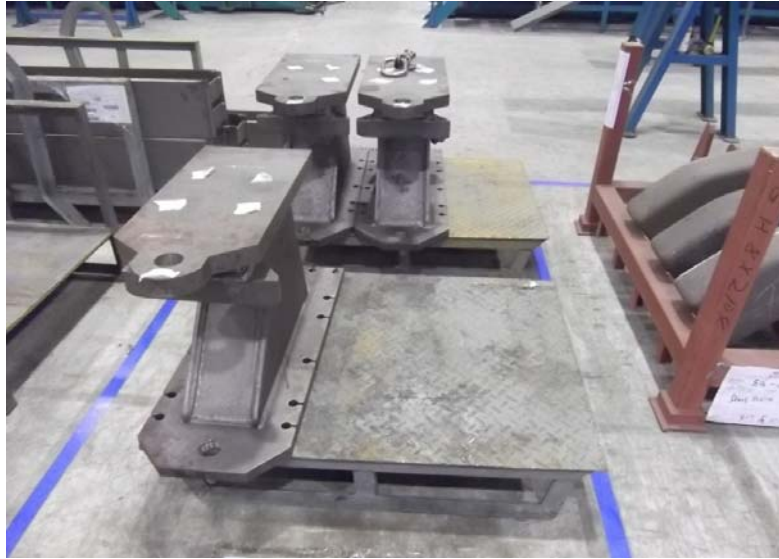
Figure 3. Bolster resting on current rack design.
