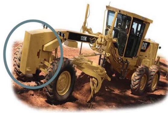
Figure 2. Bolster shown on motor grader.
