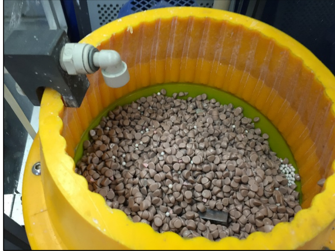
Figure 5: Edge sample being mass finished
