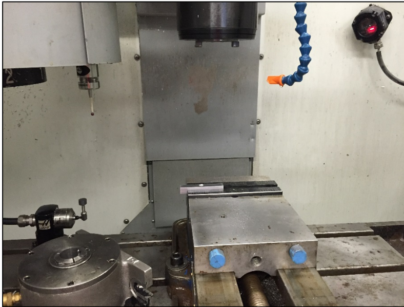
Figure 4: Edge undergoing milling operation
