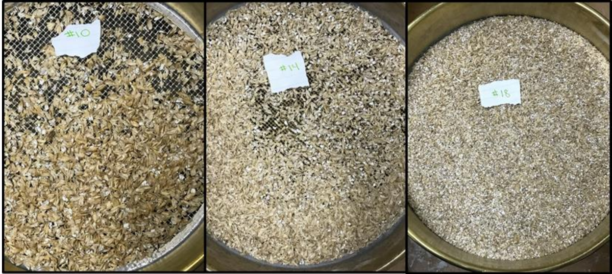
Figure 4.11: Sieve #10, #14, and #18 with Roller Gaps 1.7 mm, 0.7 mm, and 0.6 mm
