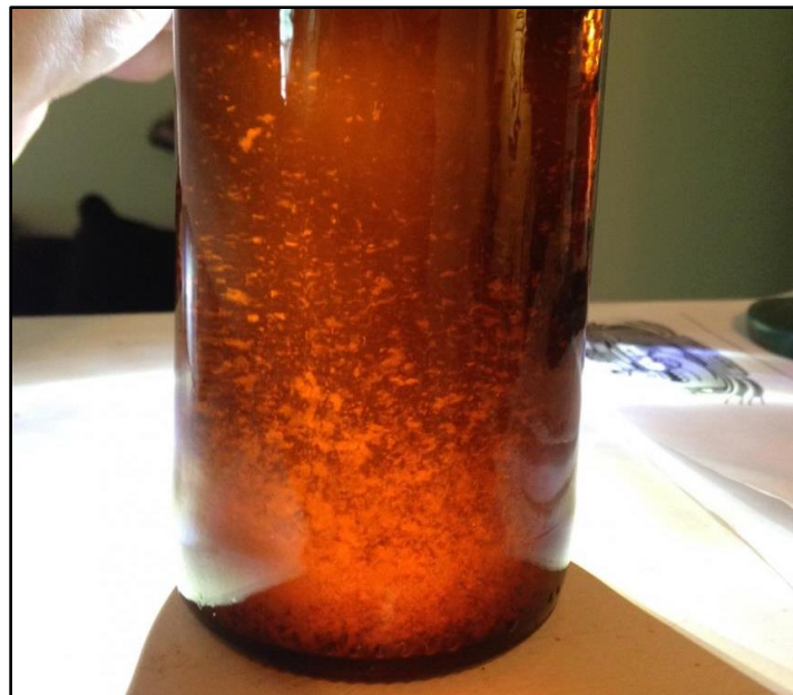
Figure 2.2: Suspended Solids in a Beer Bottle 12
