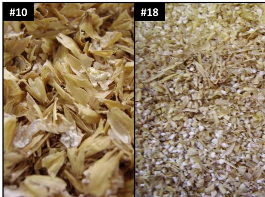
Figure 4.12: Buhler Group Pictures of the #10 and #14 Screens After Sifting (Photo provided by Roger Scheel)
