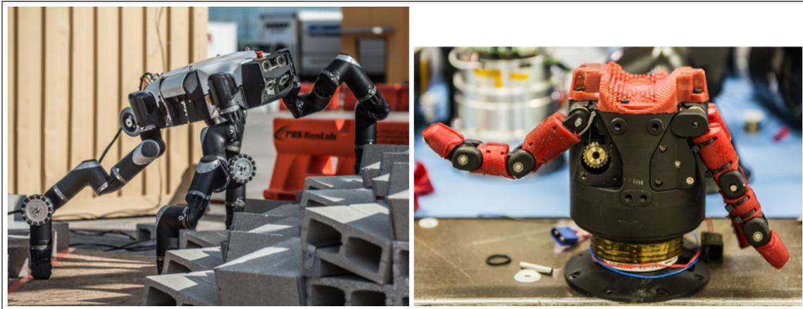
Figure 2.2: RoboSimian traversing uneven terrain at the 2015 DARPA Robotics Challenge (left). The versatile gripper (Right) had under-actuated digits and a palm designed to support the weight of the robot [14]
