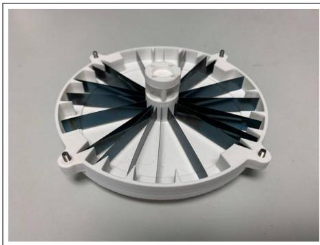
Figure 3.5: An open BENE module. The leaf springs are arranged like spokes from a central hub and jam with the geometric extrusions when bending.
