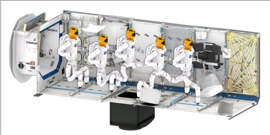
Figure 2.3: Without using its arms, R2 can navigate the ISS by anchoring onto the handrails (right) [24].
