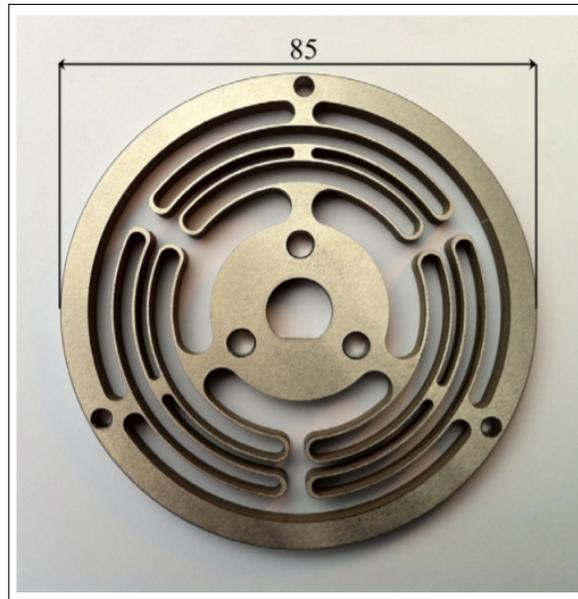
Figure 3.4: A bidirectional torsional spring developed for use in SEA for knee assistance. The spring has a 85mm diameter and is made of VACO 180T (maraging steel 300), which puts the production cost at several hundred dollars [22].
