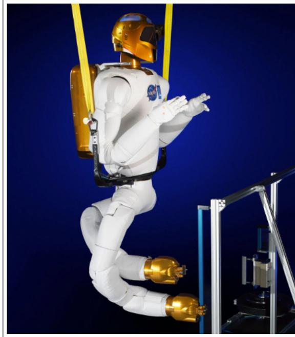
Figure 1.3: Robonaut 2 showing its manipulation limbs and locomotion limbs, the latter of which are seen anchoring it to the hand rails of the ISS [23].
