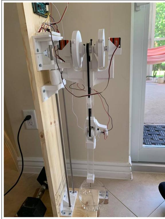
Figure 4.2: The control test experiment setup, which features the load-lifting end effector and the load reservoir. Here the hip is constrained by the additional brackets mounted behind the hip joint.
