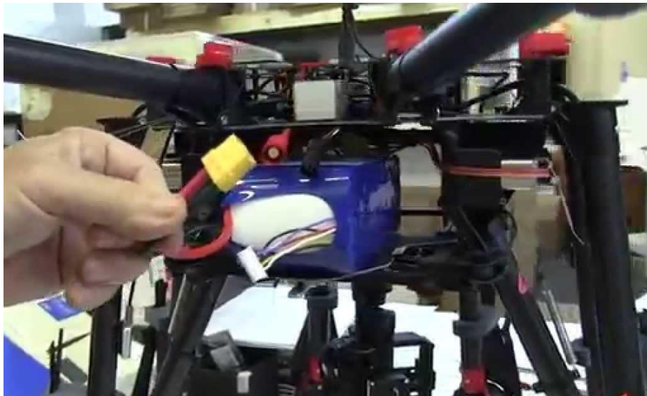
Figure 3 Battery Mounting Point
