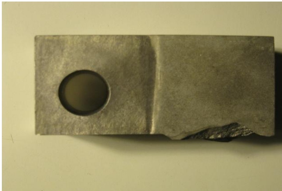
Figure 9: Test Piece After Hydrofluoric/Nitric Acid Etch
