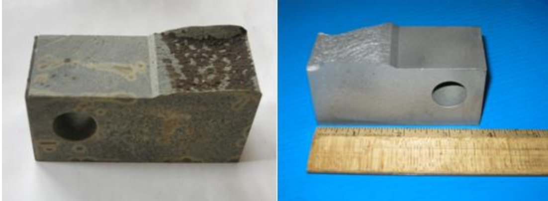
Figure 4: Two Sample Test Pieces at Different Stages (Sample on Right after Heat Treatment and Sample on Left after Grit Blasting)
