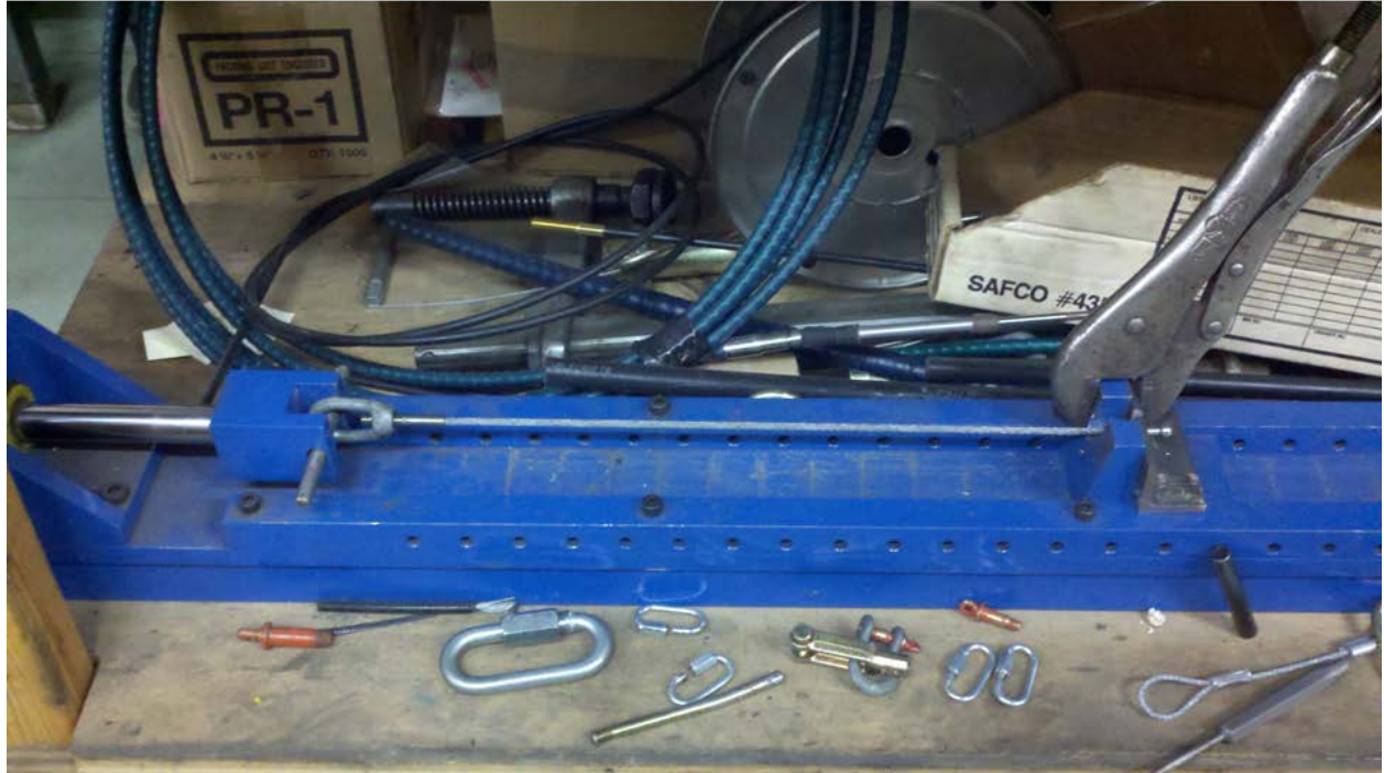
Figure 121 - Tensile Testing Setup
