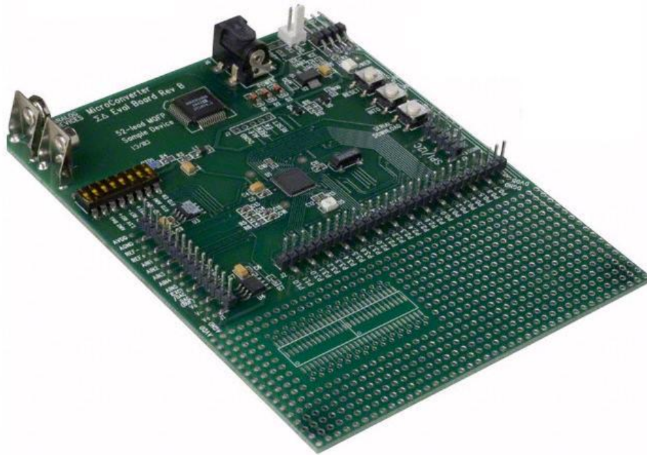
Fig.3-4: (Analog Devices ADuC845 Evaluation Board) 24
