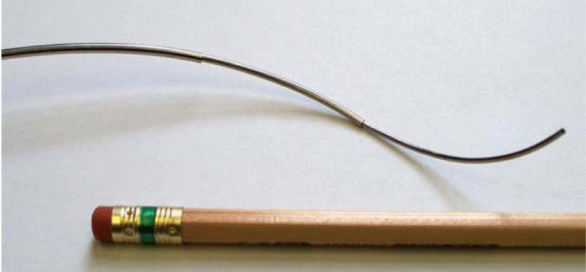
Figure 2.6: Example of a steerable concentric-tube needle with three segments (from Rucker, 2010).
