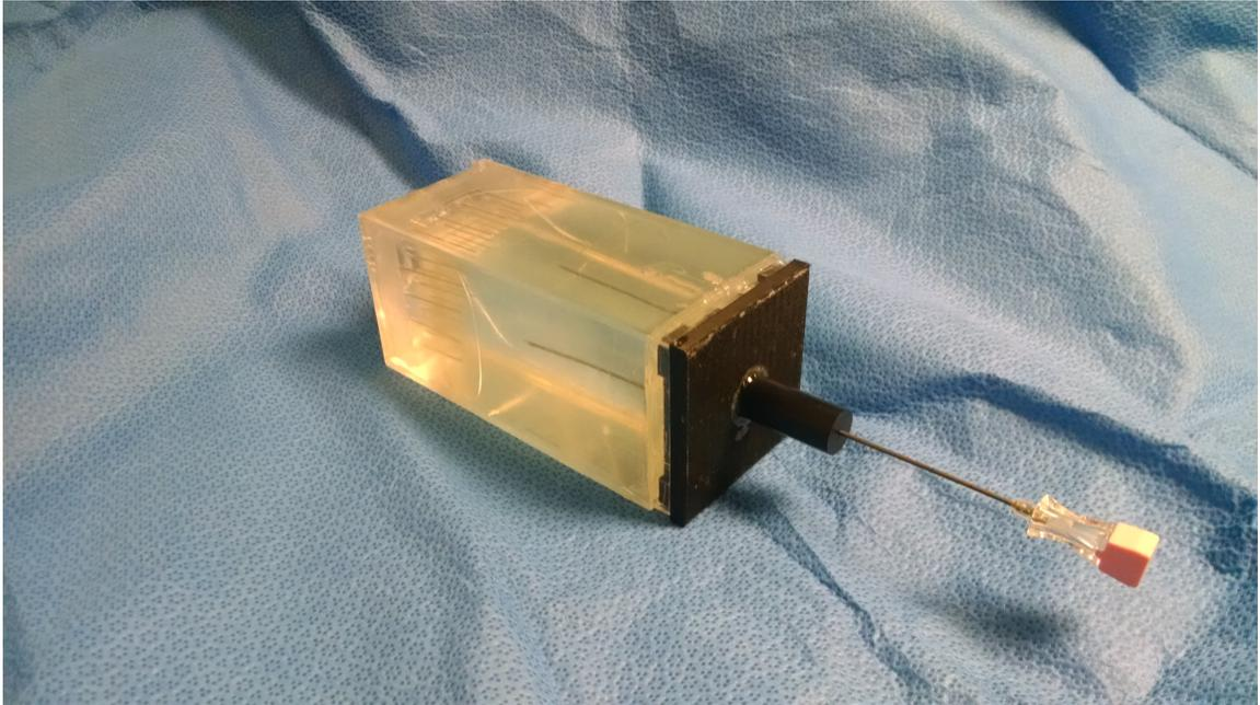
Figure 4.3: Example tissue phantom with the needle alignment frame and biopsy needle.
