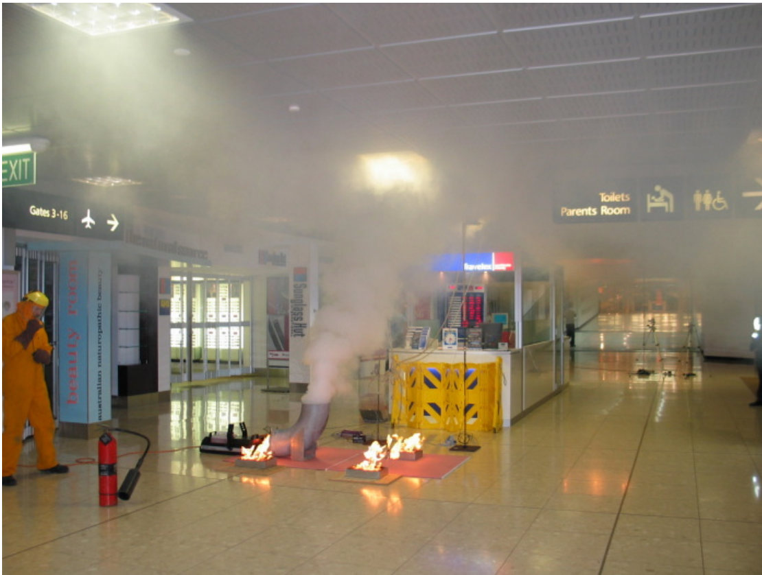
Figure 23. Test fires and instrumentation station 2 during the test.
