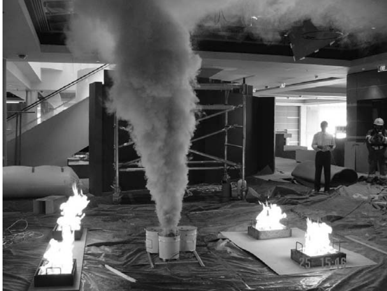
Figure 1. Typical Hot Smoke Test Layout using smoke canister.
