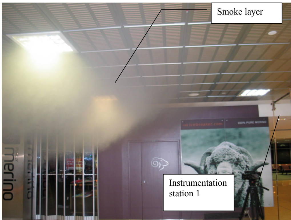
Figure 18. Location of instrumentation station 1 in regard to the smoke layer during test 1.
