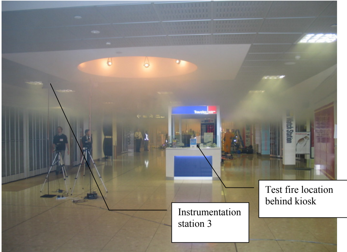
Figure 26. Location of instrumentation station 3 in regard to the test fire looking west to east.
