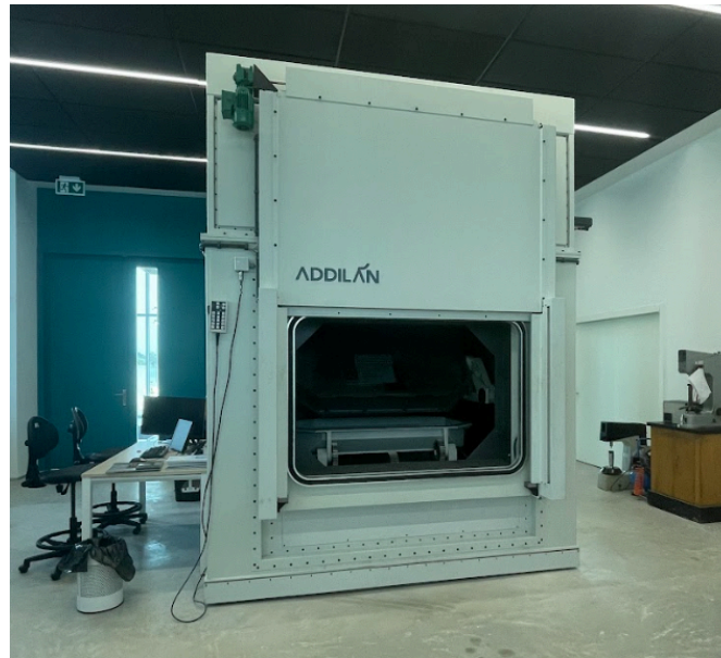
Figure 1: WAAM Machine in the Smart Manufacturing Lab at the University of Cádiz
