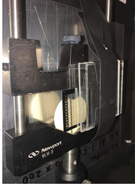
Figure 29: Imaging setup on FP-11 (ASTERIX) with scatter rejecting collimator, scattering medium, and the PSI resolution grating.
