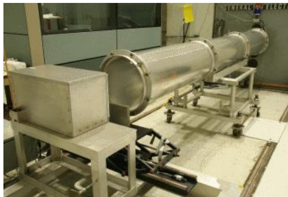
Figure 7: Cadmium lined evacuation chamber with decrease pressure for beam collimation.
