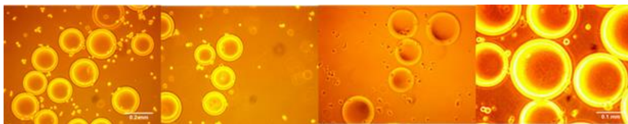
Figure 30: Microscope images of the microcarriers in the second Wave bioreactor run. From left to right, hour 1, hour 2, hour 3, day 1. All scale bars shown are 0.2 mm in length (Images 1-3 taken at same magnification)
