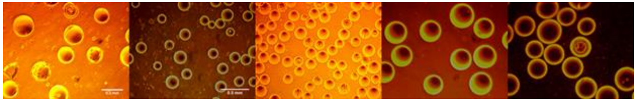
Figure 31: Microscope images of the microcarriers in the second Wave bioreactor run. From left to right, day 2, day 3, day 3 (spinners added), day 6, and day 9. First scale bar shown is 0.2 mm in length and second is 0.5 mm (images 2-5 taken at same magnification)
