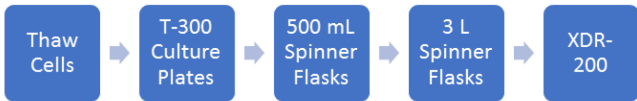
Figure 42: Final Design of Seed Train to the XDR-200
