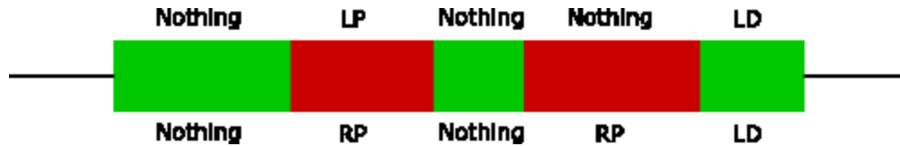
Figure 27: A timeline of rewards given to Roboxer. The coach's moves are shown on top while Roboxer's moves are shown on the bottom. Green indicates the time when a positive reward was being given while red indicates a negative reward.
