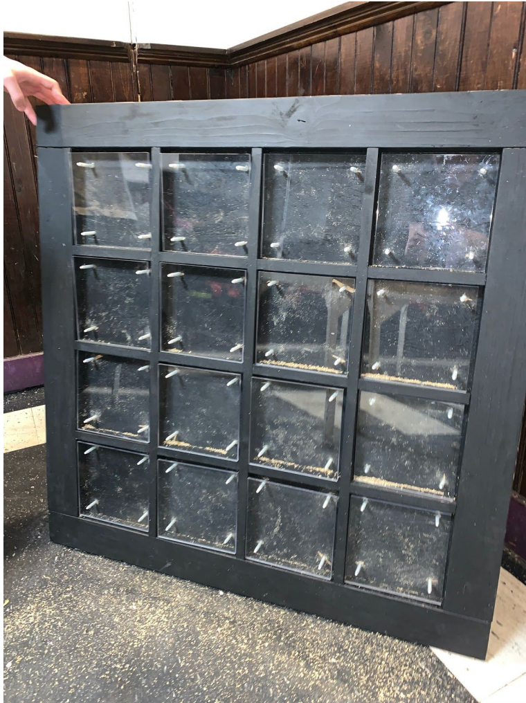
Figure 13: Grid and Backing, Drilled and Painted
