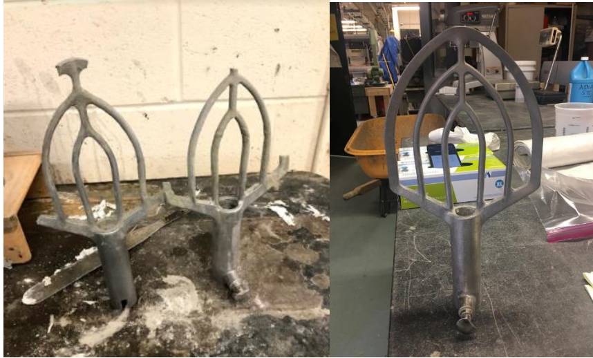
Figure 6: Broken paddles from the Hobart 20 Quart Commercial Dough Mixer and intact paddle
