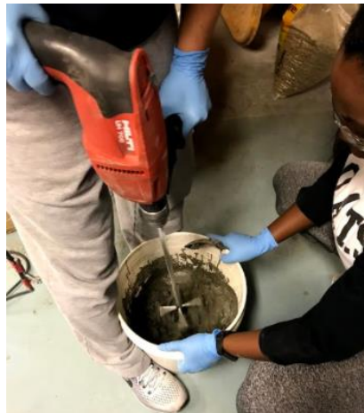
Figure 7: New mixing setup with a hand held electric drill and a mixing paddle
