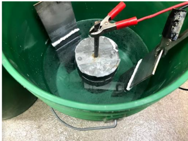
Figure 4: Corrosion test setup that consists of two steel plates, the concrete sample and a salt water solution
