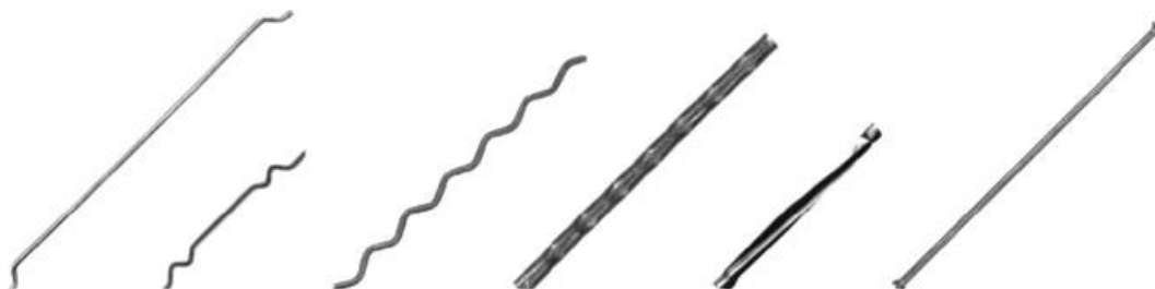
Figure 2: Different types of steel fiber deformations; hooked end, irregular, crimped, stranded, twisted, and paddled. Image courtesy of Holschemacher et al. (2010)
