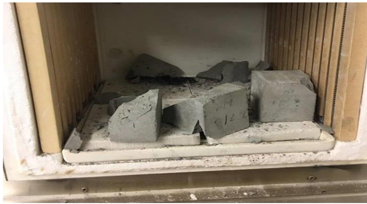
Figure 14: Three 2 in. (5.08 cm) steel fiber cubes samples after exposure to heat
