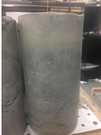
Figure 3: The initial samples showing the segregation. The light grey is the fly ash and the dark grey is the reacted cement and water.
