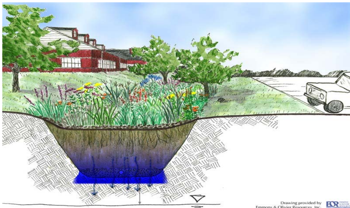
Figure 2-11: Cross Sectional View of Rain Garden (Source: Emmons and Oliver Resources, Inc., Oakdale, MN)
