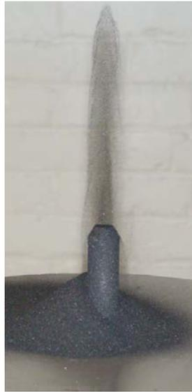
Figure 4: An instantaneous photograph showing particle injection and collection in the pan
