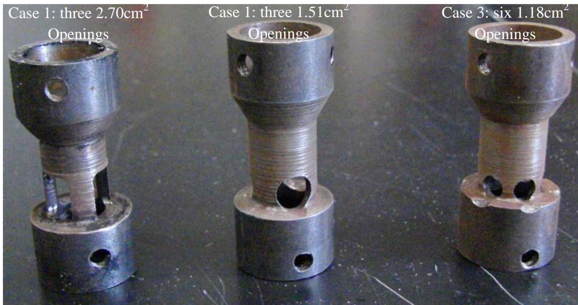
Fig.A.1-2: Middle Sections of the Novel Dust Injector
