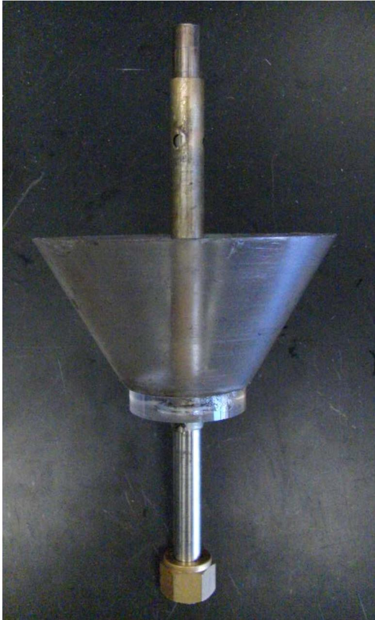
Fig. A-1.5: Burner with 60° Cone Feeder
