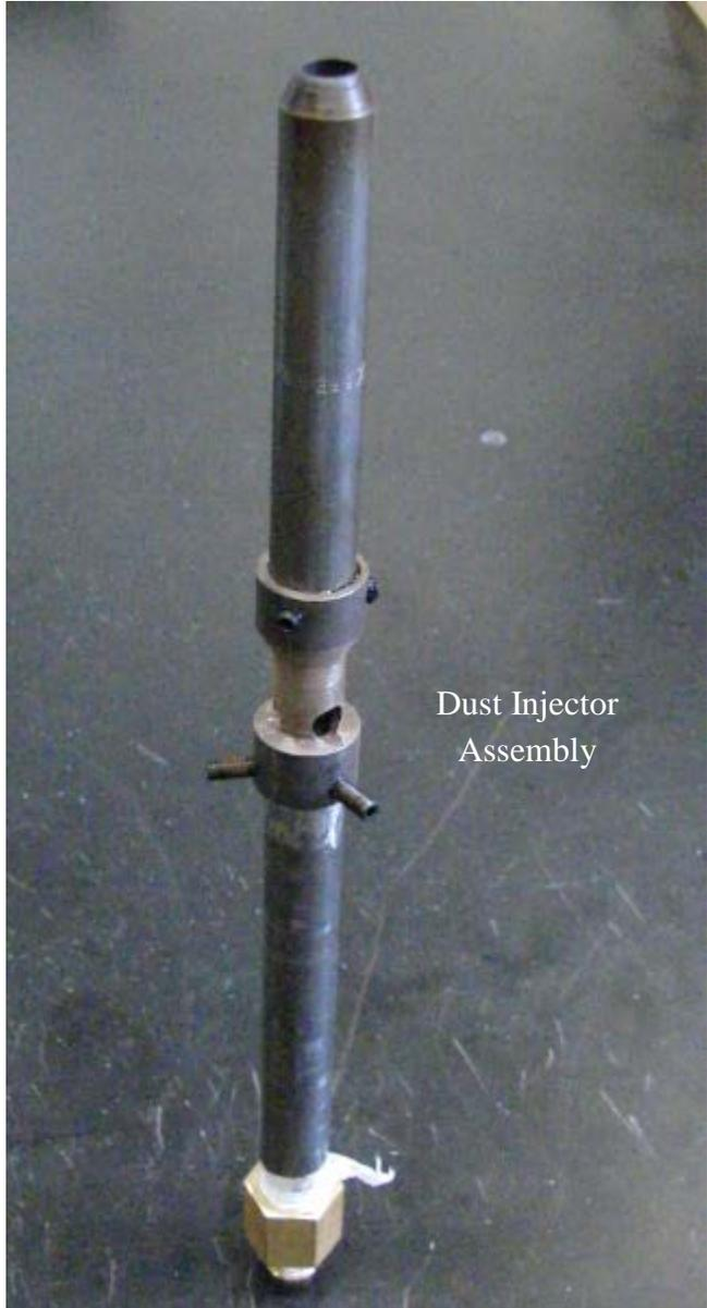
Fig.A.1-3: Dust Injector
