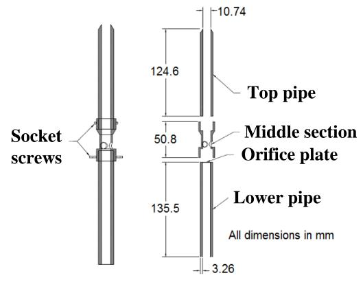
Figure 1: Solid particles injector
