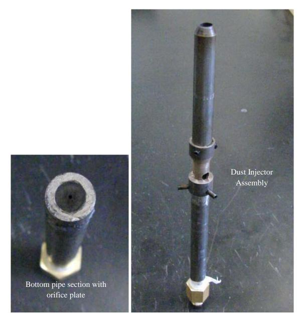
Fig.A.1-3: Dust Injector
