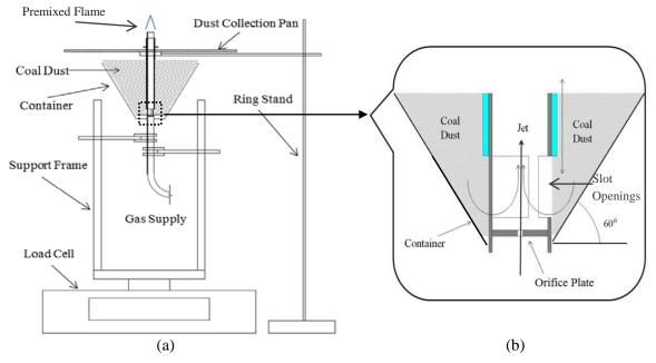
Fig. 2: Experiment apparatus: (a) dust burner and the weighing assembly; (b) the details of the dust entrain mechanism
