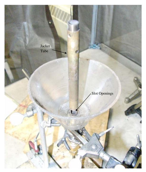
Fig. A-1.6: Burner Assembly
