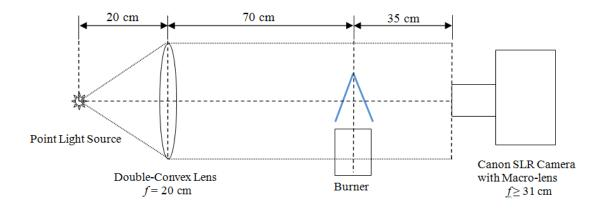
Fig. 3: Shadowgraph set-up
