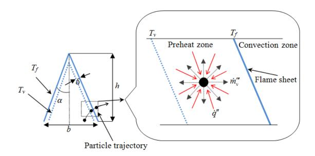
Fig. 5: Illustration of parameters involved ( $\dot{q}''$  is the heat flux from flame to the particle;  $\dot{m}_v'''$  is volatile release rate per unit volume of the mixture;  $T_f$  is fame temperature;  $T_v$  is coal devolatilization initiation temperature;  $\delta$  is the thickness of devolatilization zone;  $\alpha$ is the cone half angle; *b* is the burner diameter; *h* is the cone height.)
