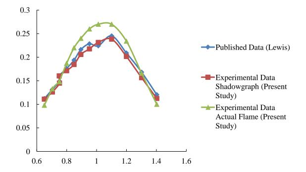
6. S<sub>u</sub> (gas only) with Equivalence Ratio Ranges from 0.7 to 1.4
