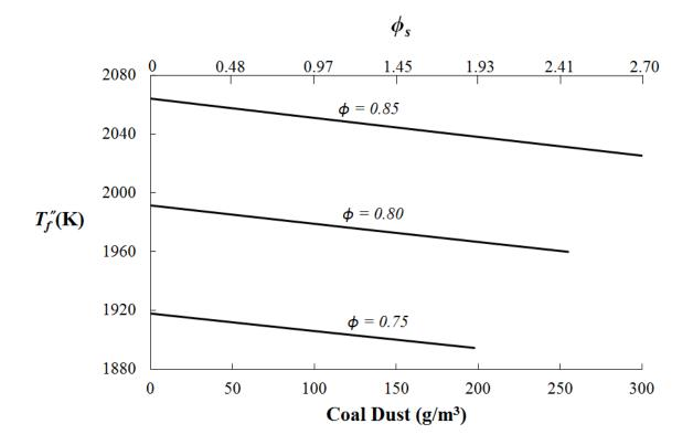
Fig. 7: The flame temperature based on the heat sink effect of coal particles at 75-90 µm
