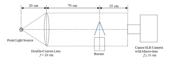
Fig. A-1.9: Shadowgraph Setup
