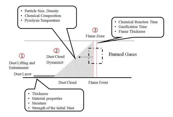
Fig.1: Dust explosion process
