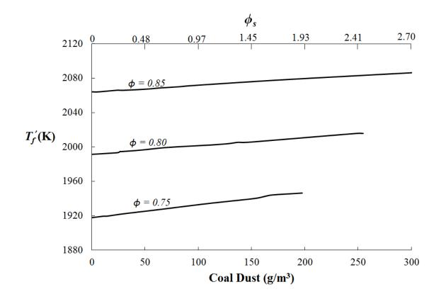
Fig. 6: Adiabatic flame temperature based on  $\phi$  with additional gaseous fuel released from coal particles in the size range of 75-90 µm.
