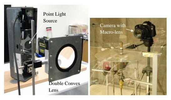
Fig. A-1.9: Shadowgraph Apparatus
