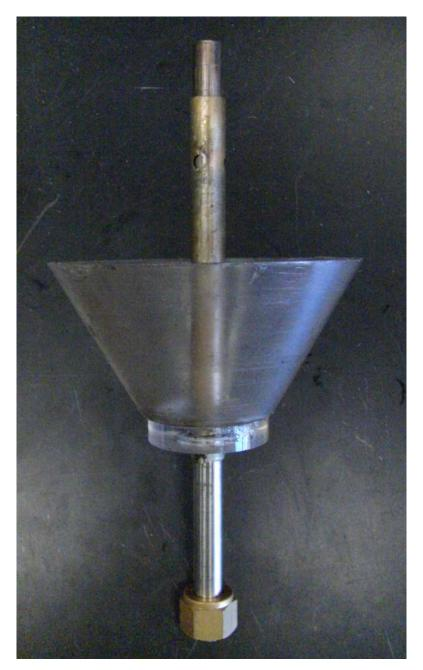
Fig. A-1.5: Burner with 60° Cone Feeder
