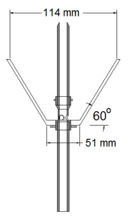
Figure 2: Injector with particle feeder
