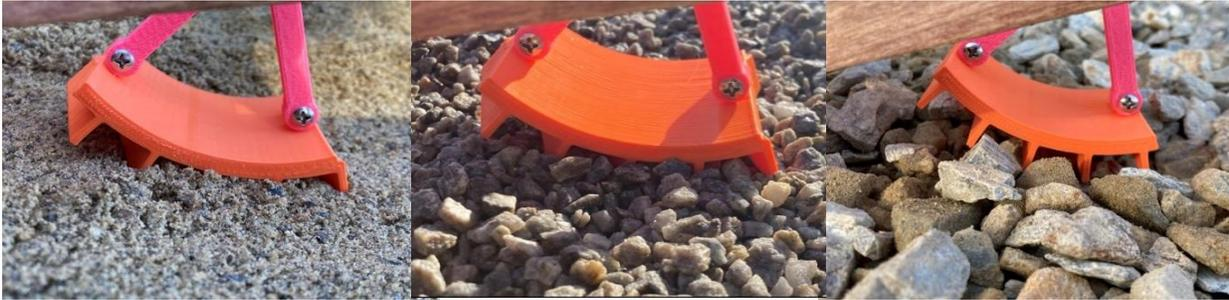
For the sake of consistency in the data collection, a single team member was responsible for pulling the scale at a constant rate to the best of their abilities for all the trails. The force displayed on the scale was recorded just before the tread slipped out from its grip in the gravel. Table 4 below shows the results of this experiment in units of newtons.
