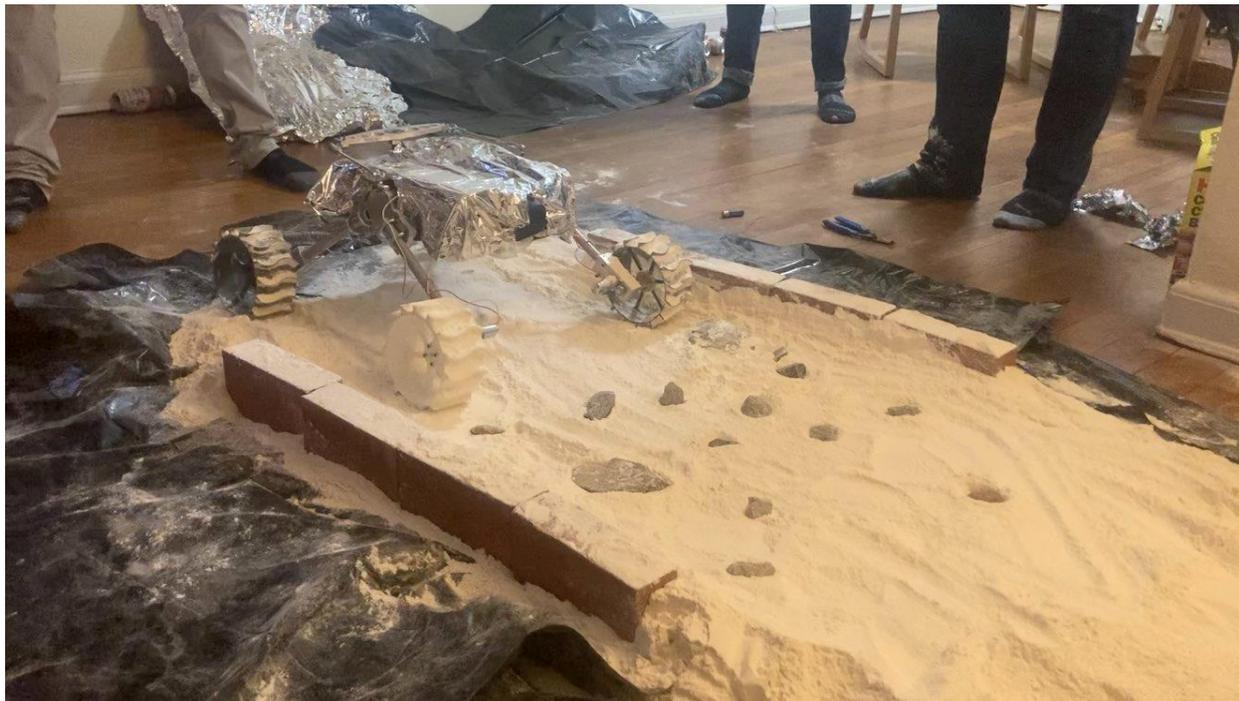
**Figure 49:** The micro rover navigating the secondary drivetrain test mid-traversal over a small rock.
