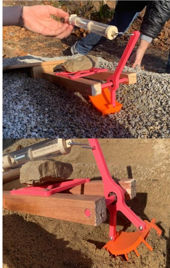
The testing rig also featured a larger platform towards the back of the pivoting component that allowed a weight to prevent the rig from moving backward as the scale was pulled. Three trials were conducted for each tread design and length at each different size of gravel. A sample of a wheel tread going through each size of gravel is shown in Figure 46.
