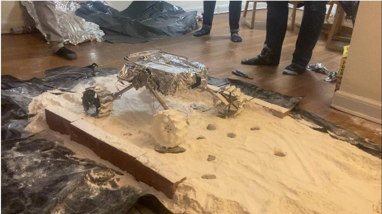
After the successful navigation of both the initial and secondary drivetrain test, a third, and final test was required to ensure the stability of the drivetrain before moving on to more difficult tests. This final test saw the addition of two bricks laid side by side in front of one of the wheels, with the intent of forcing the Rocker-Bogie system to actuate. Once again, the rover traversed the obstacle successfully.
