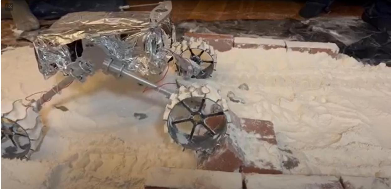
The rover was also tested to see the max step obstacle size it could traverse. For this test, bricks were stacked to replicate a set of stairs. The rover was able to climb up the bricks giving the team confidence in its ability to easily traverse over small obstacles that it may face on the moon.
