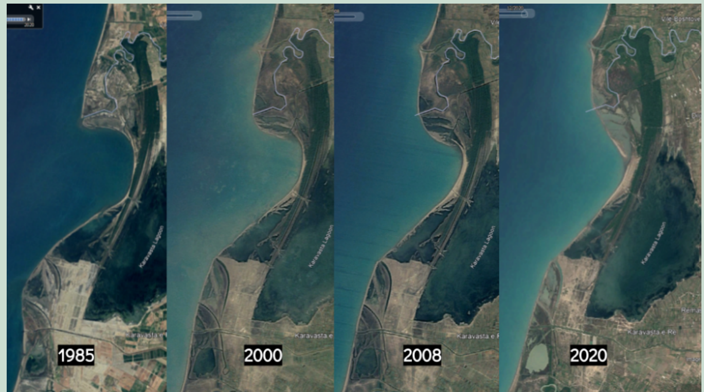
Figure 4.15: Changes of the coastline during the last 30 years. Along with the coastal changes, the Shkumbini River diverted its course in 1992, shifting its mouth further north. (Google Earth, 2022)
