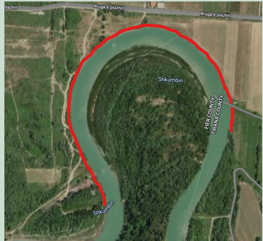
Figure 4.4: One of the specific riparian forest buffer sites. The red line shows where the tree line would be planted.
