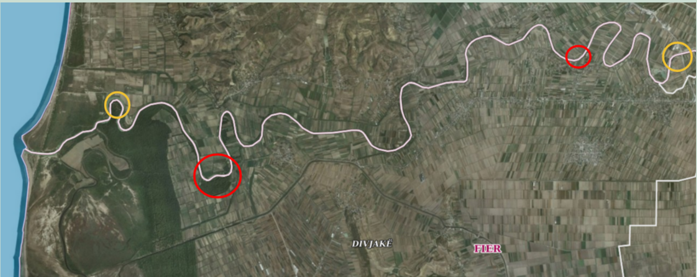
Figure E.3: Location of proposed riparian forest buffers (yellow circles) and proposed rock walls (red circles) along the Shkumbini River
