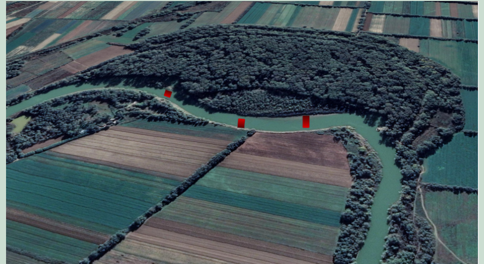
Figure 4.11: The location proposal to place 3 rock walls at a bend in the Shkumbini River
