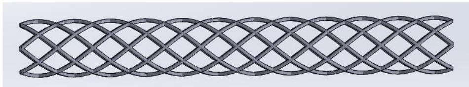
*Figure 1: An example CAD model of a stent.*
