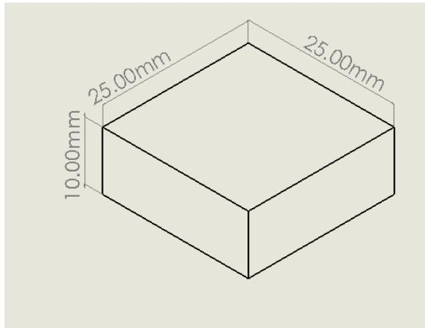
**Figure 6: CAD drawing of the samples.**
