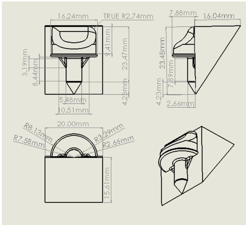
**Figure 7: CAD drawing of the modified knee implant.**
