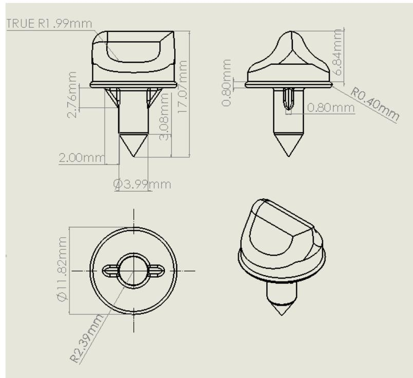
**Figure 4: CAD drawings of a knee implant.**
