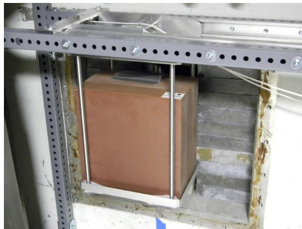
Figure 13 - The solid water positioned in front of the collimation tube. The bag containing the dosimeters is held to the solid water blocks by tape.
