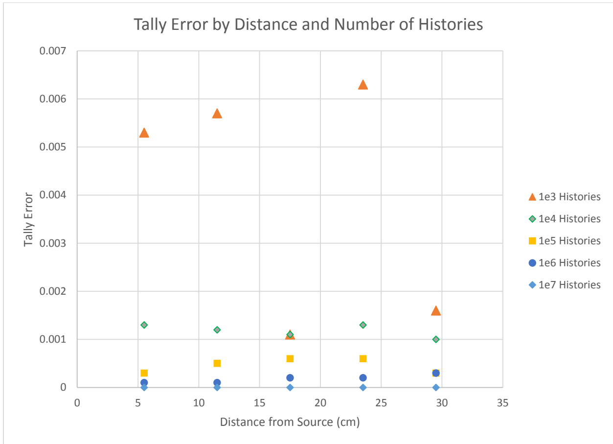
Figure 14 - A plot of reported error at various tally distances by number of histories taken. As the number of histories increases, error decreases. No error is reported at any distance when 1 \times 10^7 histories were simulated.
