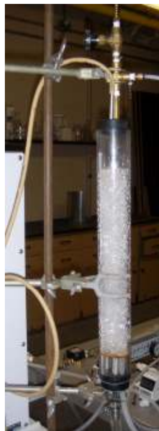
Figure 6: Miniature absorption column used in data collection for absorption/reaction system
