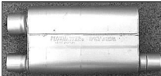
Fig. 26. Case 3 Flowmaster 80 series Cross Flow muffler (Flowmaster, Inc., 2009).
