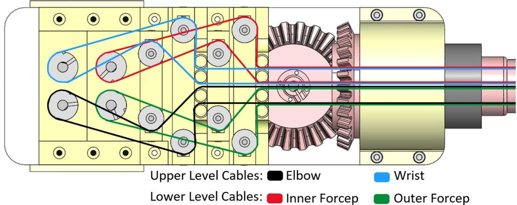
Figure 4.6: Top view of cable paths on base plate
