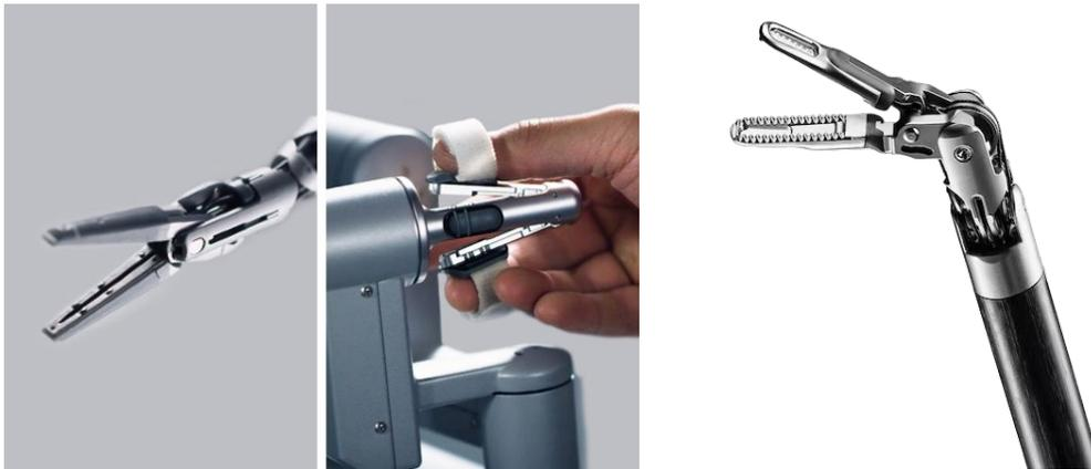
*Figure 2.1: The left figure depicts the full da Vinci endo wrist next to its control mechanism at the operation station. The right figure shows a closeup view of the toolhead for the da Vinci endo wrist. [12]*
