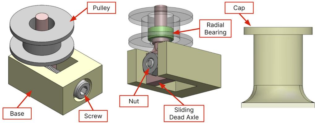
Figure 4.5: Tensioner (left) and idler (right) design
