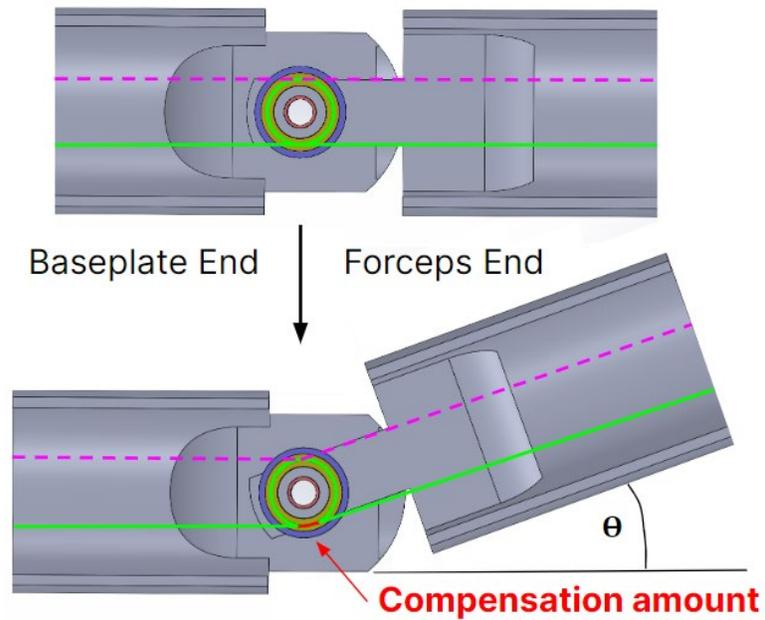
Figure 5.2: Visual representation of cable length compensation in the elbow joint.
