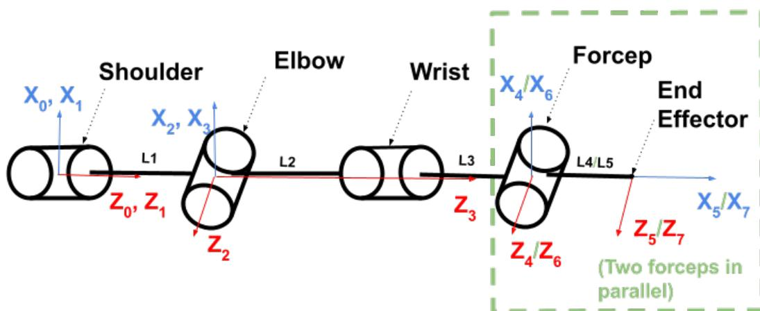
Figure 4.2: Kinematic diagram of the instrument.
