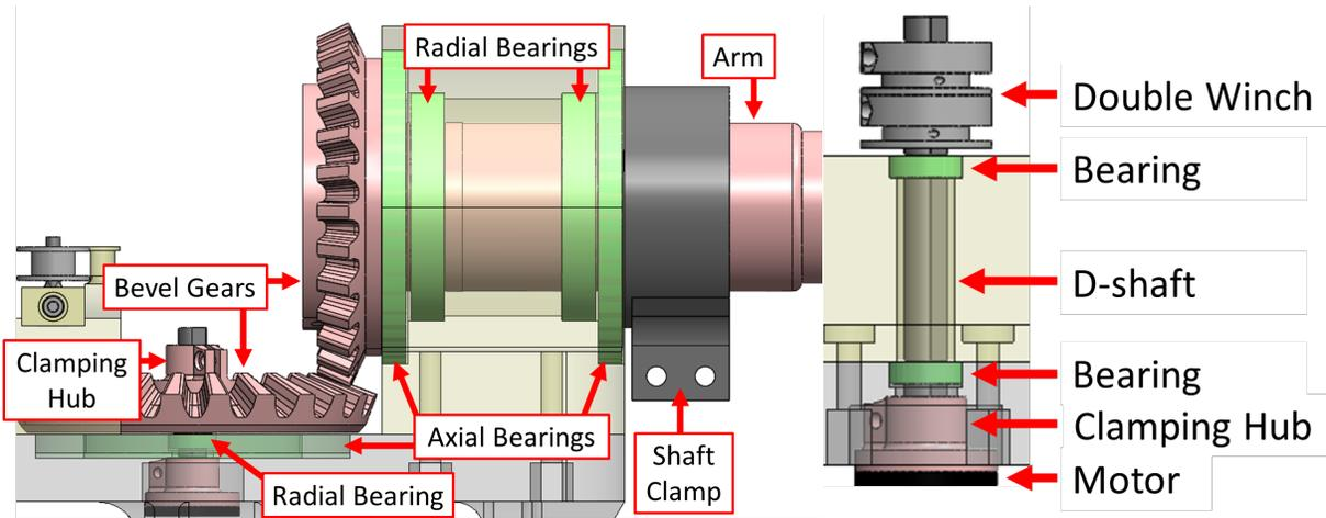
Figure 4.4: Side views of shoulder (left) and driving shafts (right)
