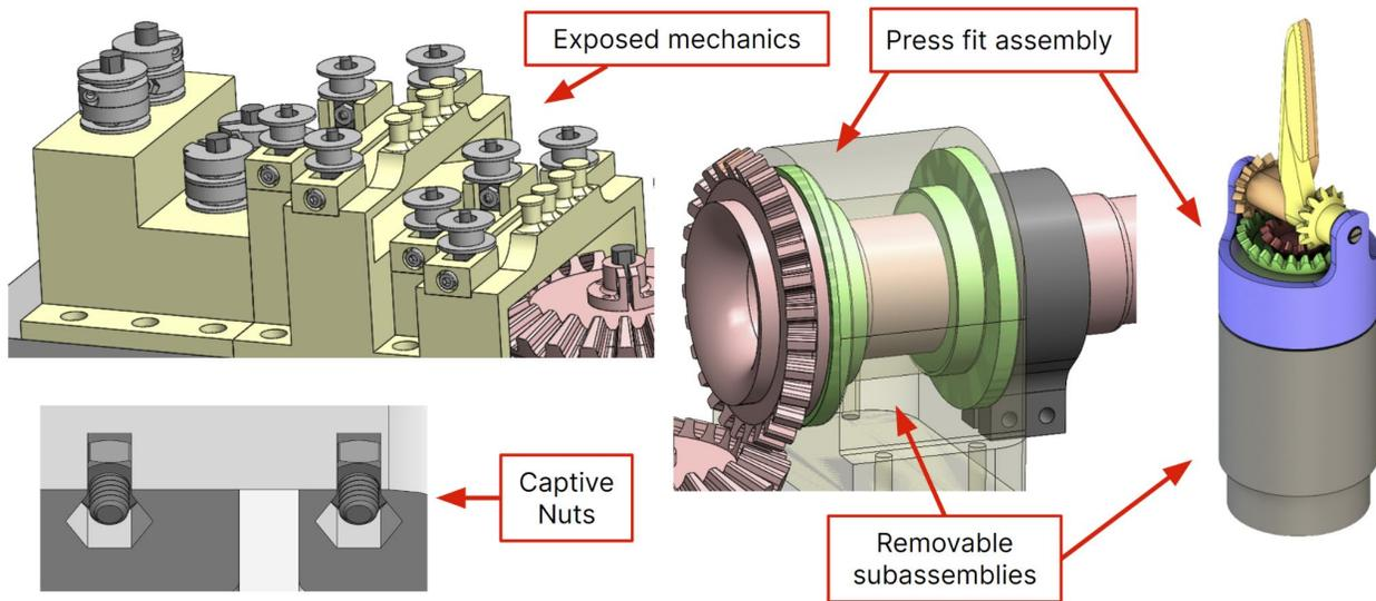
*Figure 4.13: Examples of Design for Manufacturability (DFM) integrated into the instrument's design*
