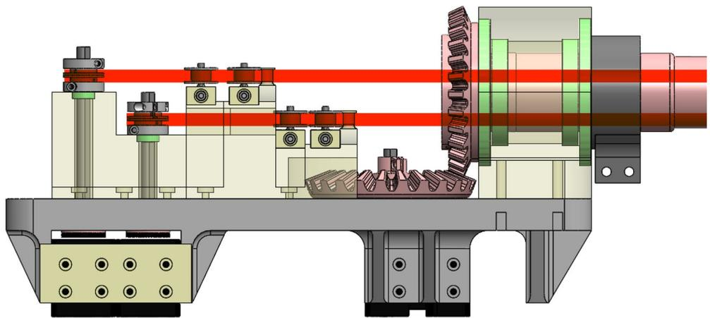
Figure 4.7: Side view of cable paths on the base plate
