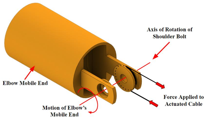
*Figure 4.10: Isometric view of the mobile end of the elbow.*
