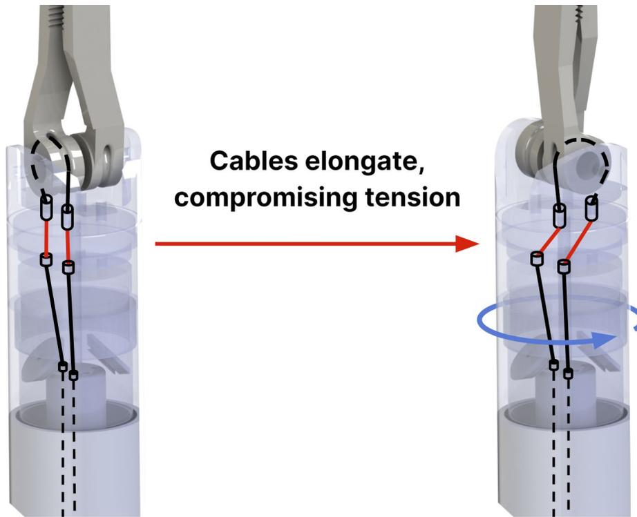
*Figure 4.12: Cable elongation problem, illustrated when the wrist rotates from a properly tensioned position (left) to an elongated position (right)*
