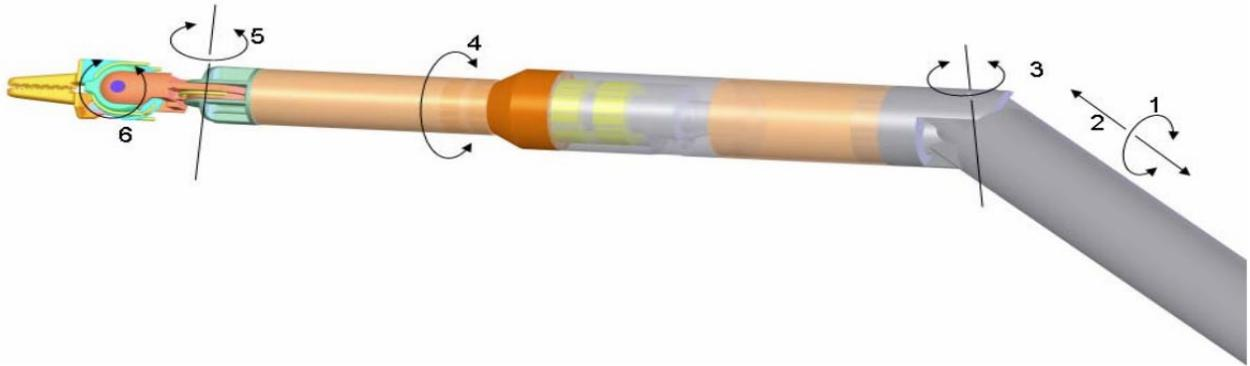
*Figure 2.4: 6-Degree of Freedom Cable-Driven Robot [14]*
