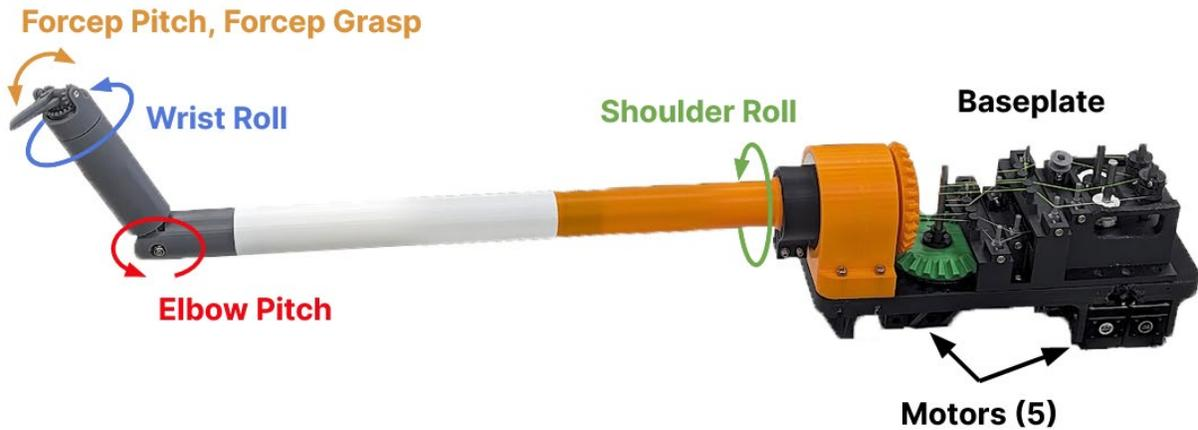
Figure 4.1: Five DoFs instrument prototype with its unique kinematic layout that includes both shoulder and wrist roll.
