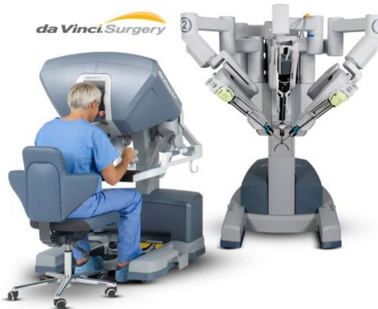
*Figure 2.2: The figure above shows the full da Vinci surgical system. The left figure depicts the remote base station where the surgeon operates. The right image shows the full multi arm system with attached toolheads. [12]*
