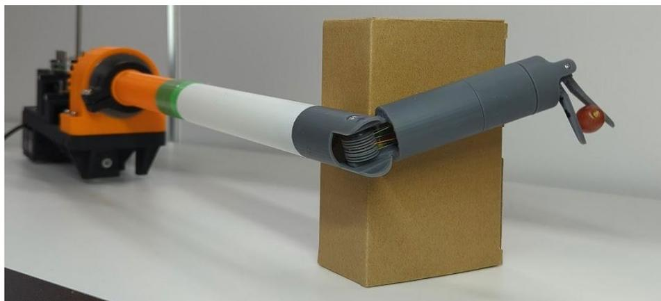
*Figure 6.4: Device manipulating a grape behind an obstacle.*
