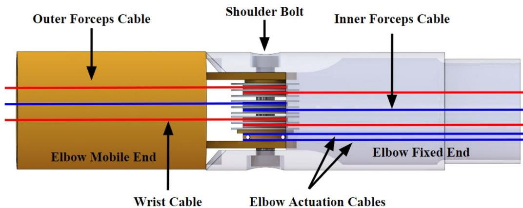
Figure 4.9: Elbow top down view with transparent fixed end. Pulleys in the center for organization of the cables needed to actuate the wrist and forceps.
