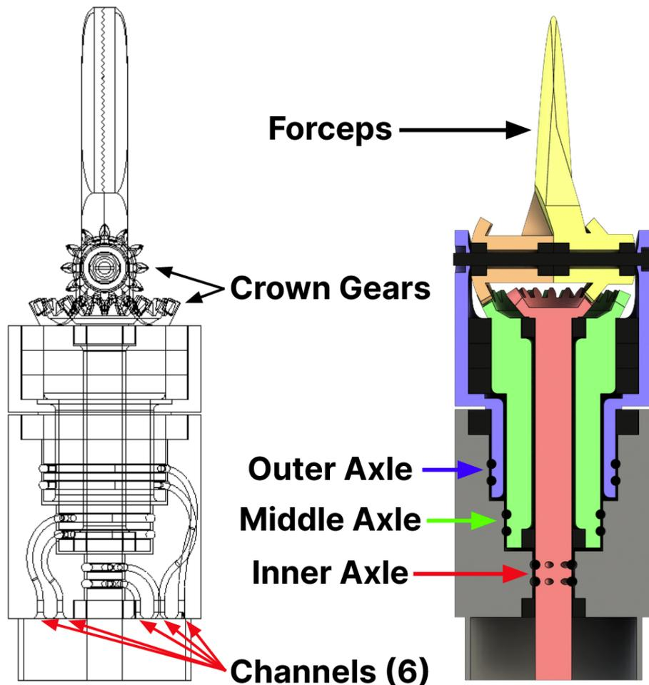
Figure 4.11: Wireframe side view (left) and cross section front view (right) of wrist roll and forceps.
