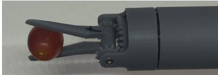
*Figure 6.3: Wrist roll compensation test with grasp.*
